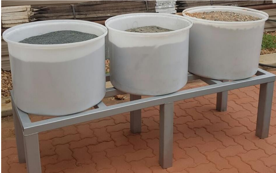
Figure 6: Leach Drum setup. Natural Rainfall set in TNG Alice Springs warehouse yard.
