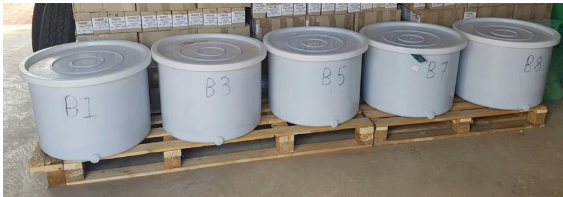
Figure 5: Leach Drum setup. Simulated Rainfall set in TNG Alice Springs warehouse.
