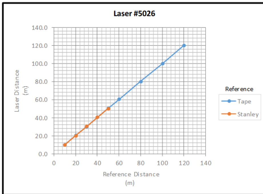
Figure 11 Calibration plot for laser #5026
