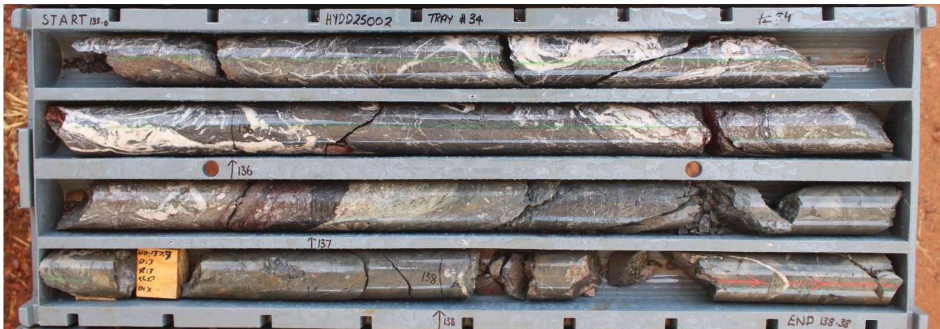
Figure 12: HYDD25002 – Tray 34 135-138.38m – showing well-developed, multi-phase quartz-carbonate vein system hosted in moderately foliated metasedimentary rocks.
