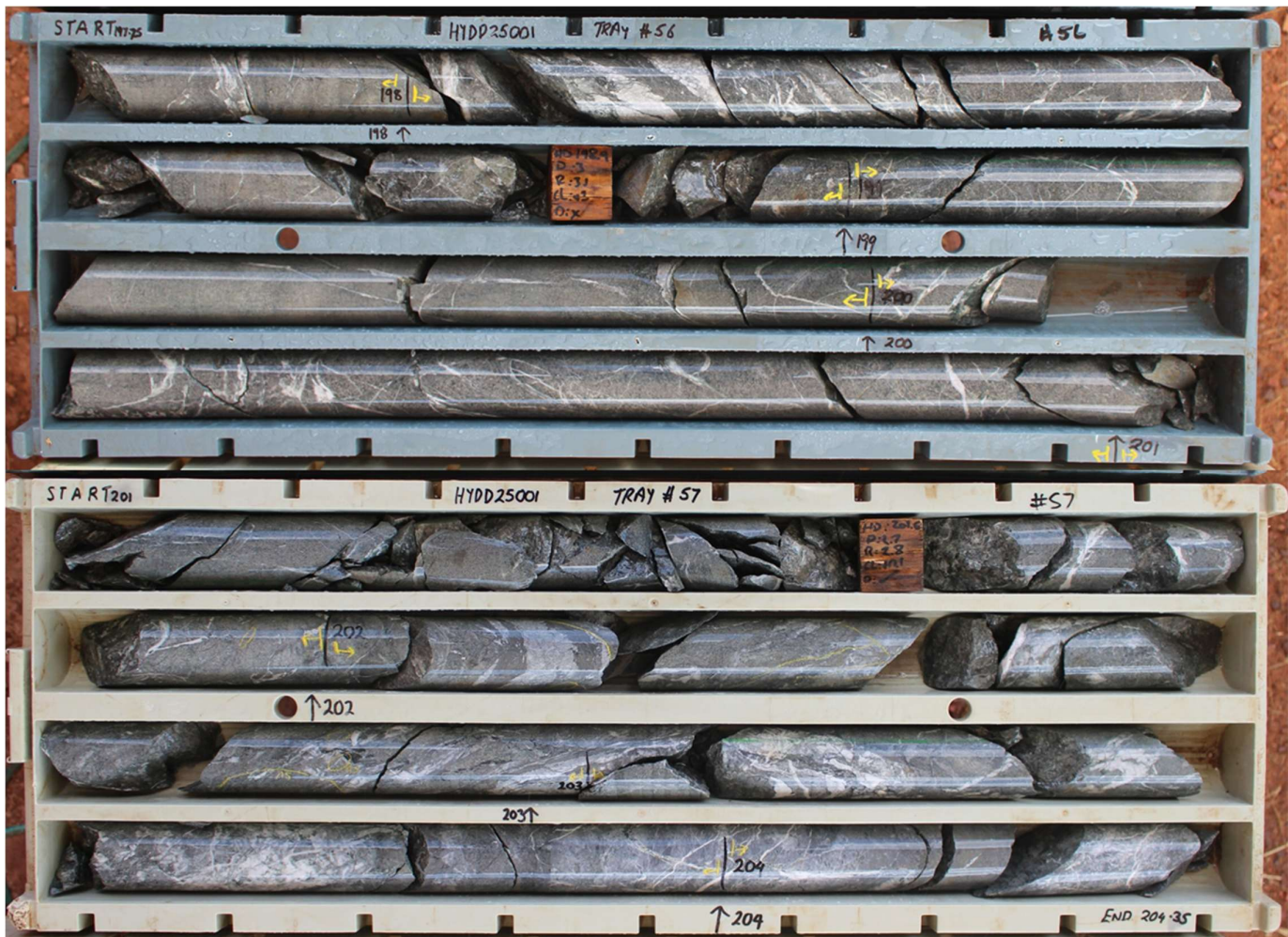
Figure 8: HYDD25001 – zone of highly veined core with moderately abundant pyrite and arsenopyrite – gold values generally 0.5g/t Au (5m @ 0.5g/t from 199m (ETW 4.5m)).
