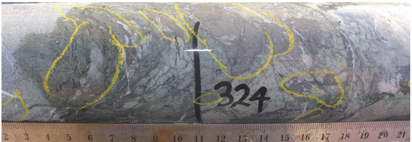
Figure 13: HYDD25002 ~324m – arsenopyrite and pyrite rich zone (323.6-324.15m – 1.44g/t Au).
