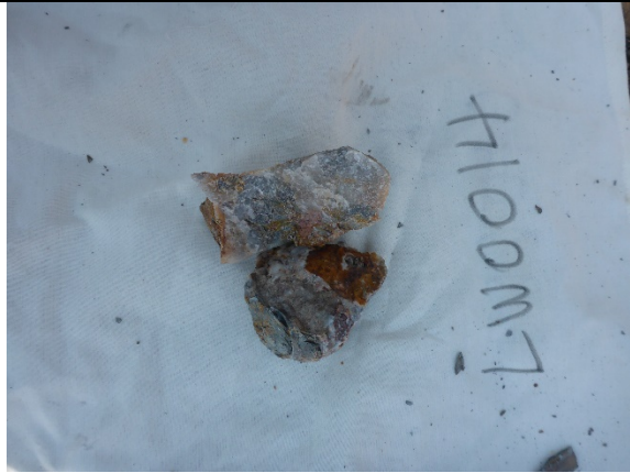
LW0014 mullock quartz with fe staining sample, 331.15 g/t Au (Grants Prospect)
