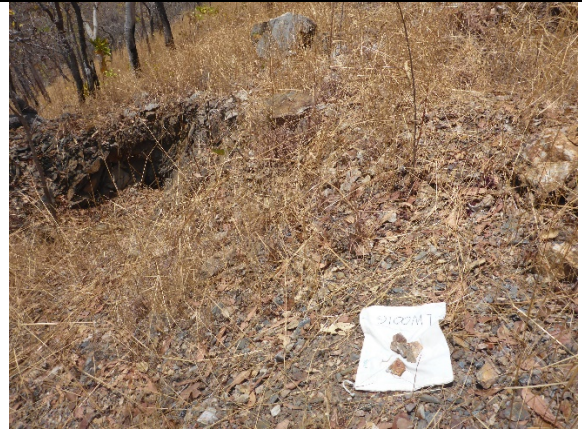
LW0016 quartz sample from small scale working on hill near Bigmouths Prospect (assayed 21.79 g/t Au)
