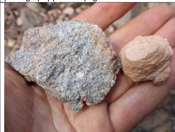
F.g granite (with quartz veining) and micaceous schist comparison
