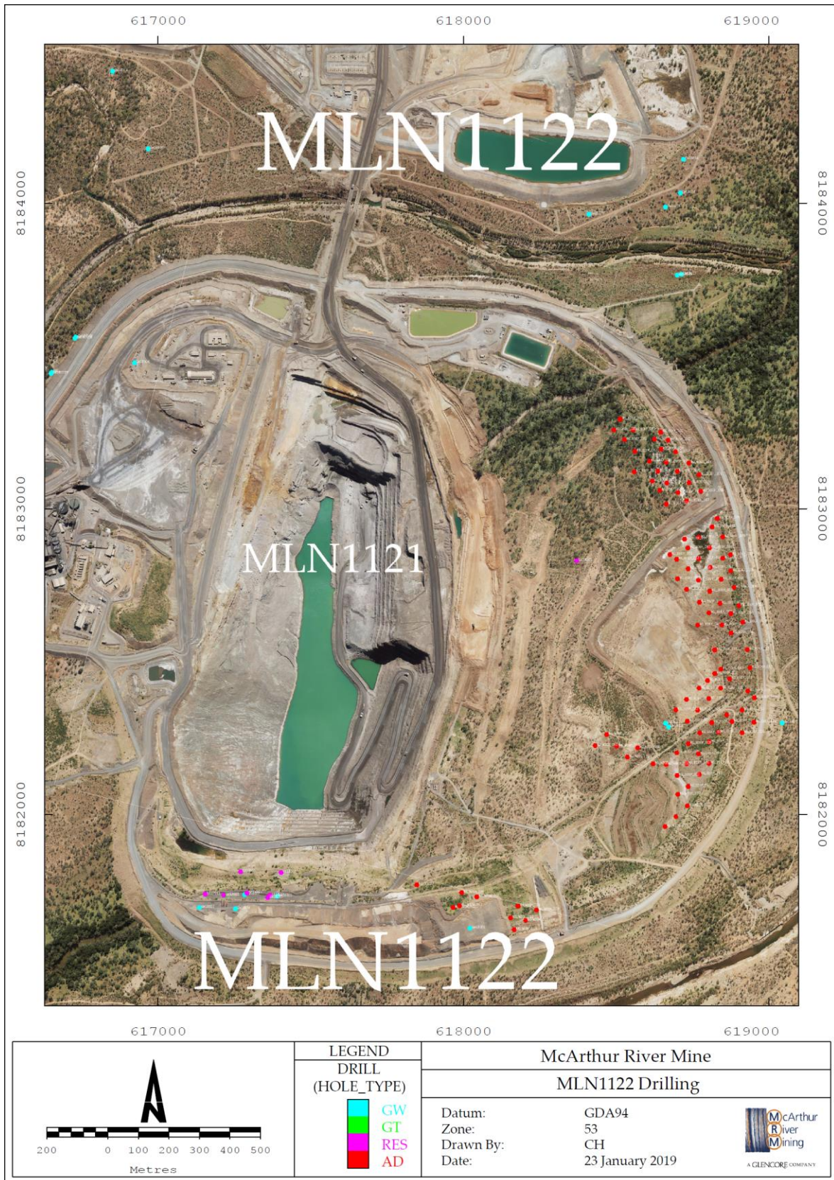
FIGURE 5. MLN1122 DRILLHOLE LOCATIONS. GW = GROUNDWATER, GT = GEOTECHNICAL, RES = RESOURCE, AD = ALLUVIUM DEFINITION.
