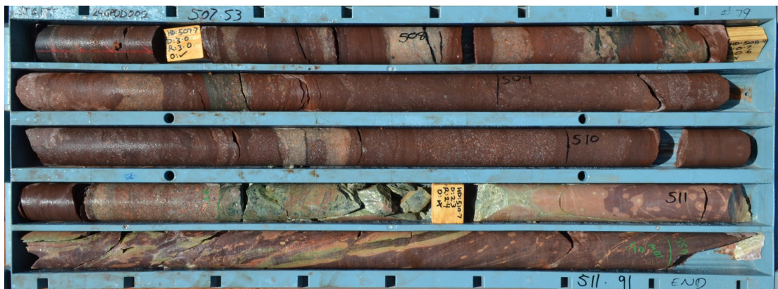
Figure 3: Drill core from 24GPDD002 showing an angular unconformity from flat-lying basin sandstones to deformed basement shales
