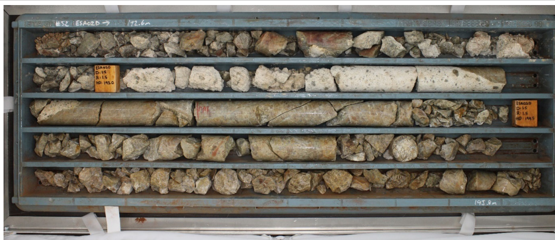
Figure 6: Drill core from ESA02D shows fault brecciation in zone of anomalous lead and silver.
