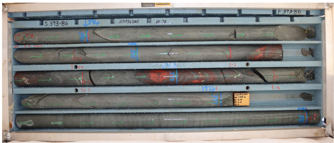
Figure 4: Drillhole 25P38D001 intersected a zone of strong magnetite with pyrite replacing jasper between 395.5 and 396.2 m.
