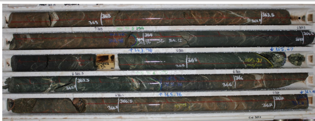
Figure 12: GFDD0002 drill core contains mineralisation within felsic intrusive and sheared contacts.
