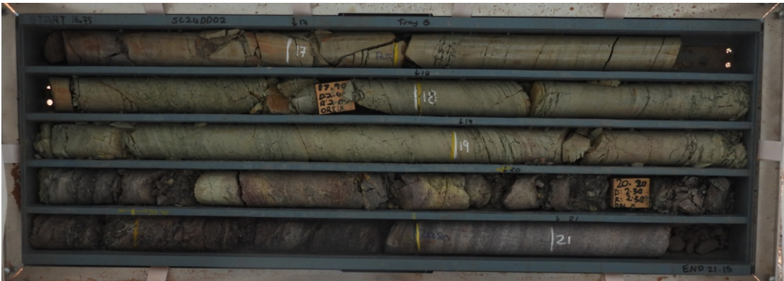
Figure 11: Dolerite at faulted contact with anomalous intercept of 2.6 m @ 280 ppm U 3 O 8 and 0.11 g/t Au from 20.4 m in SC24DD002. Future work The results support continued exploration of the Southern Comfort–Mageera linkage zone, including validation of historic drilling and further testing of the structural corridor.
