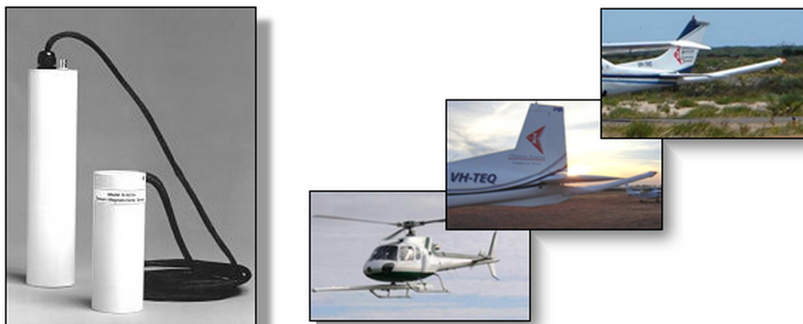
Figure 7 G822A Magnetometer and Typical Stinger Mounts
