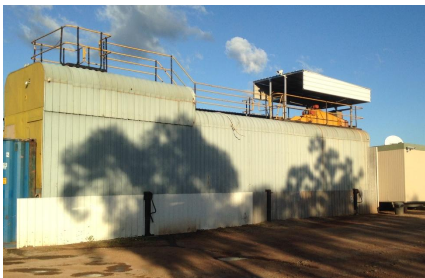
PHOTO 13: Modular Flowsort X-ray Sorter housed in a mobile caravan
