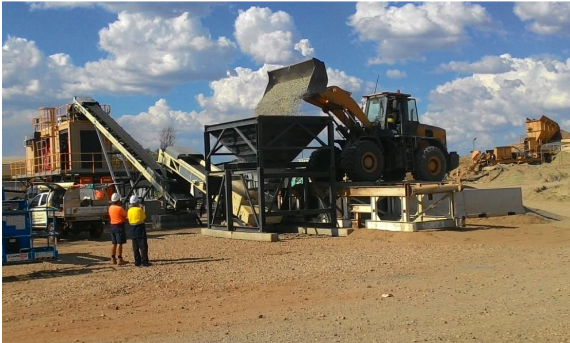
PHOTO 11: Batch feeding sized ore to TOMRA unit
