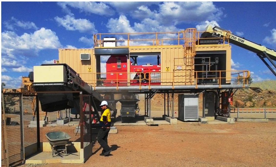
PHOTO 9: The Merlin TOMRA XRT is housed in a sea-container mounted on a raised platform when fully operational; concentrate from the TOMRA will be delivered to a hopper housed in a secured cage
