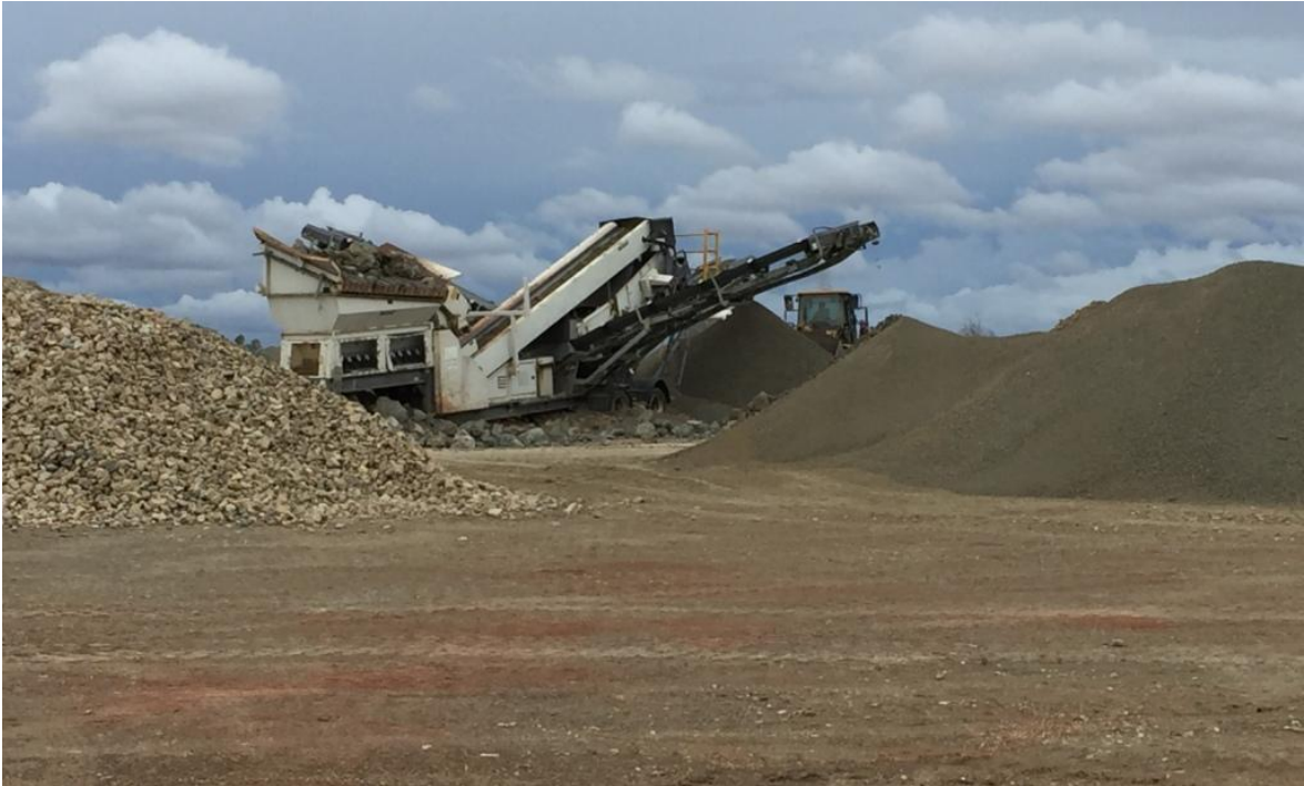
PHOTO 7: Mobile screening plant used to prepare feed for TOMRA. Feed for TOMRA was screened in three size fractions +4 to -8mm, +8 to -18mm, and +18 to -40mm.
