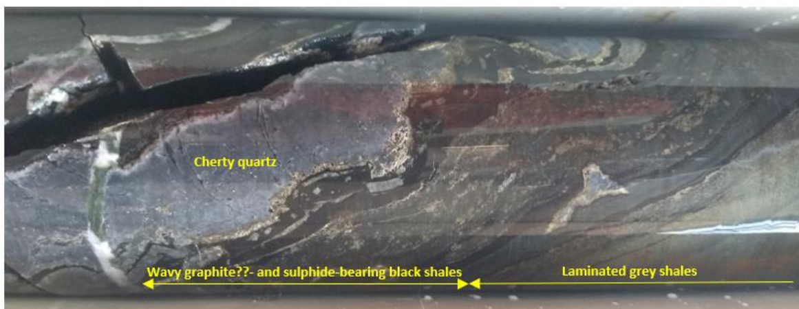
Figure 6 – Mineralised quartz vein from the Beef Bucket gold sequence in hole RRDH09.
