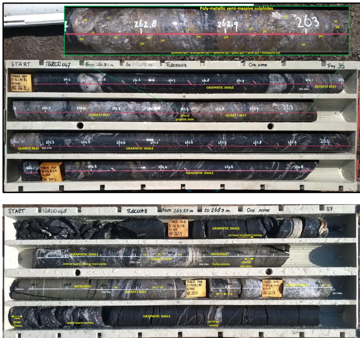
Figure 5: Diamond drill core from the ore zones for holes TGRCD047 and TGRCD048. The red line is an ori line representing bottom of hole, the white line is a cut-line.
