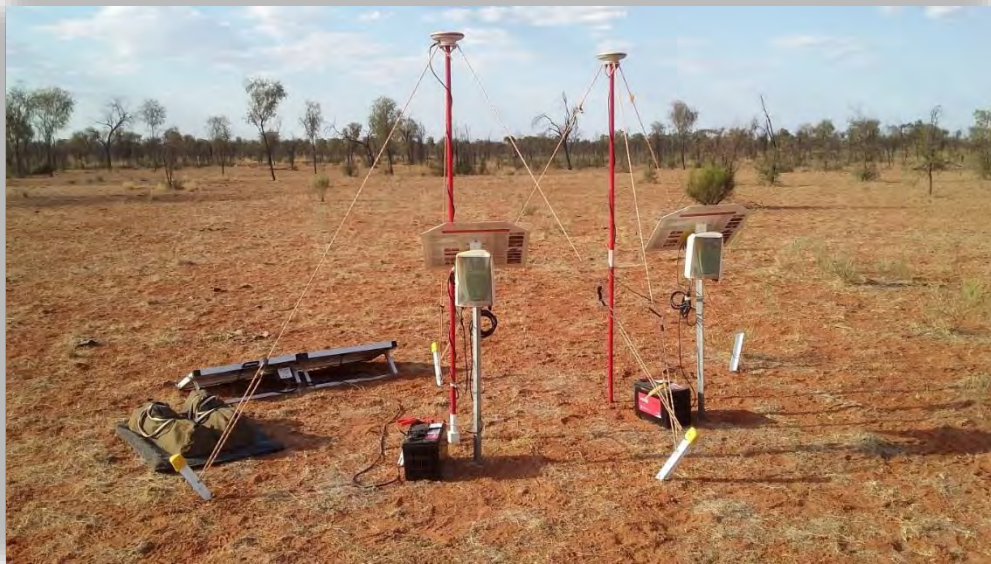
Photo 6 – A Leica GX1230 GNSS receiver set up over base 1538 with a redundant base set up nearby
