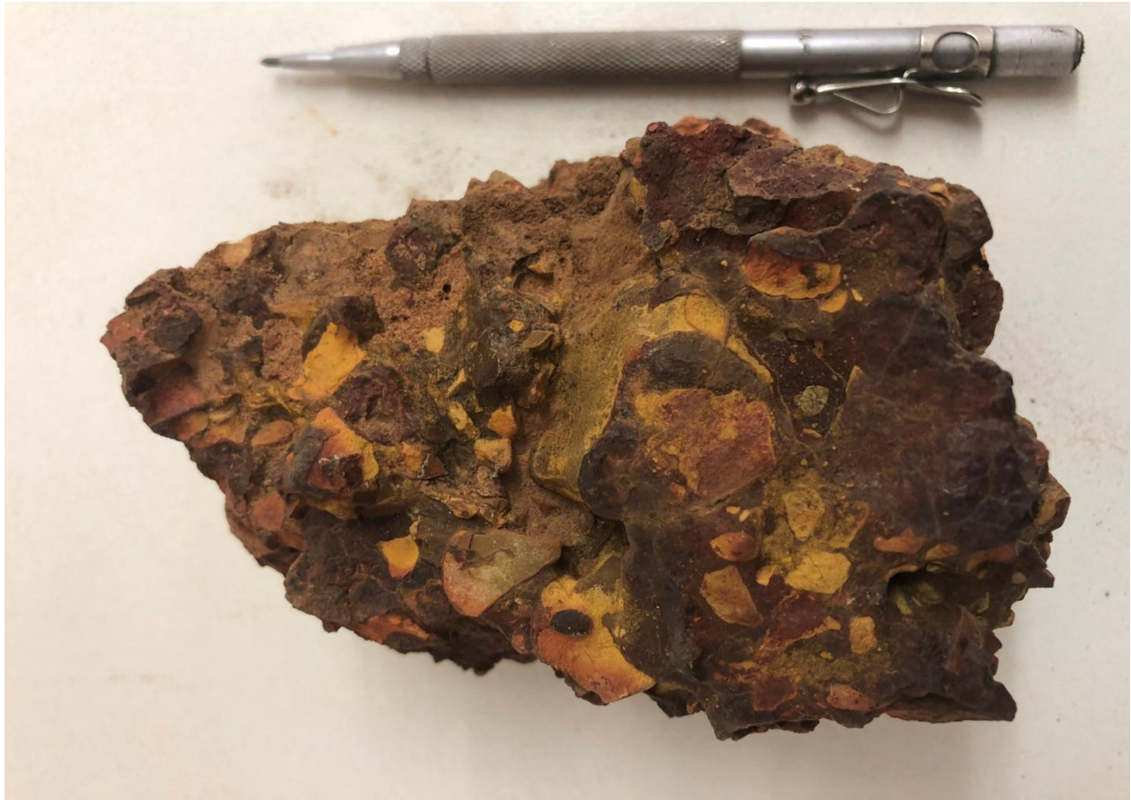
Figure 7; Laterite from the Tyson area, this sample was located in a dry cut down stream bed and it contains clasts of Ooradidgee sediment which were probably eroded into the channel at the time of formation.
