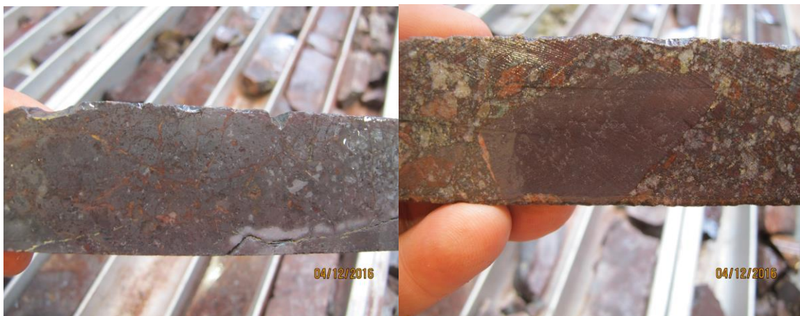
Plate 3: Mineralised interval from hole RU39, hosted within milled breccia (left), Plate 4: Mineralised interval from hole RU39, hosted within brecciated interval (right).
