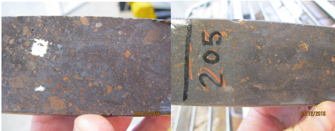
Plate 1: Mineralised interval from hole URAN1, hosted within milled breccia (left). Plate 2: Mineralised interval from hole CAR002, hosted within milled breccia (right).
