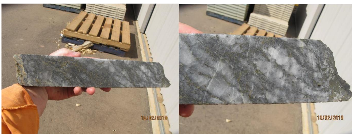
Plate 56 & 57: Core sample from 53.5-53.95 metres depth, showing quartz veining and coarse sulphides (py-cpy). This comprised part of the final sample; 17275 from 53-54 metres which was assayed at 7.7g/t Au.
