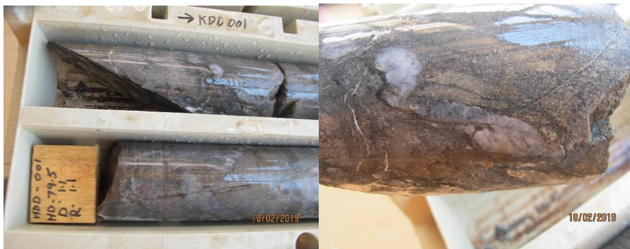
Plates 33 & 34: Core interval around 78.5 metres depth, showing small boudins within quartz veining evidence for a strong degree of ductile deformation within footwall.
