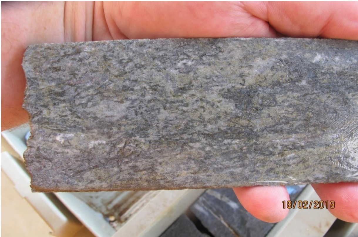
Plate 31: Core sample from 69.8 metres depth, showing moderately-altered metapsammite and lesser subhedral arsenopyrite masses.
