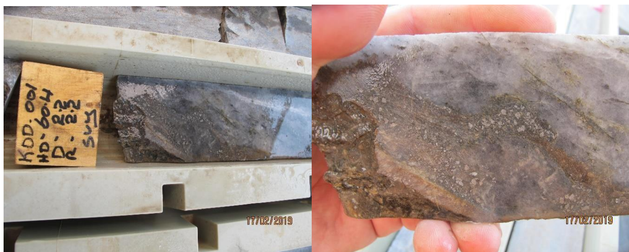
Plates 16 & 17: Core interval 60.4-50.6 metres showing coarse quartz-sericite veining which overprints earlier fabric. Coarse anhedral to subhedral arsenopyrite masses up to 2-3 mm diameter are formed/aligned with the late-stage veining, with lesser fine masses of disseminated pyrite and chalcopyrite was observed.
