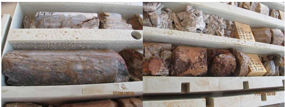
Plate 8 (left): Heavily silicified, veined and fractured core sample around 45 metres depth.
