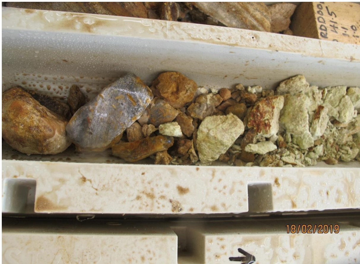
Plate 43: Heavily oxidised/chloritic clays logged to a depth of 43.65 metres which was interpreted to be a calc-silicate unit.
