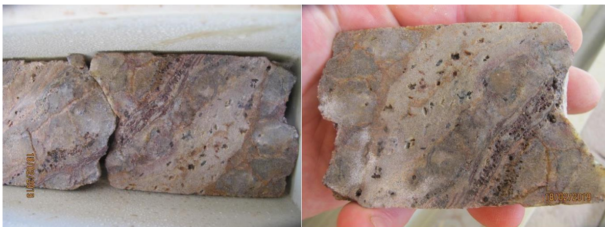
Plates 46 & 47: Core sample at start of sampling interval (depth 48 metres), showing etching of arsenopyrite masses suggesting a localised oxidation depression immediate to Hole KDD-002.
