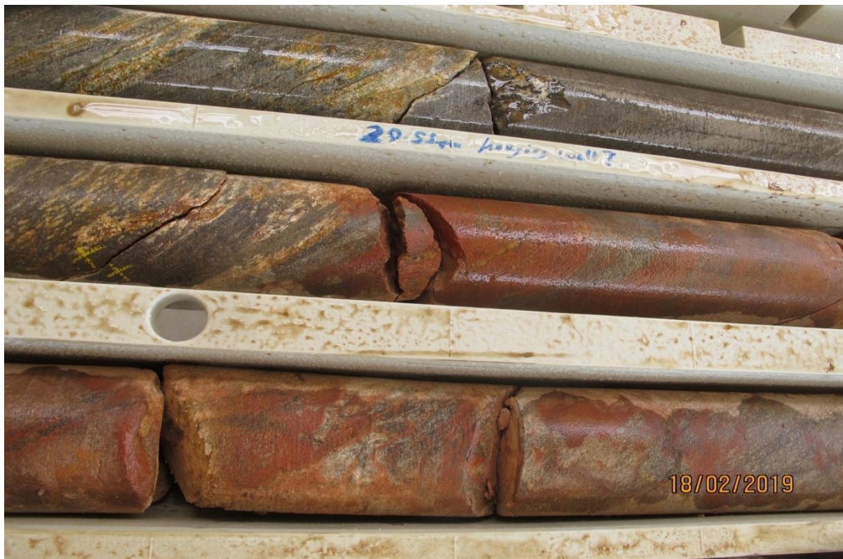
Plate 39: Start of strong haematite-mottling at 29.55 metres which was interpreted to be the upper mineralisation/hanging wall(?) contact.
