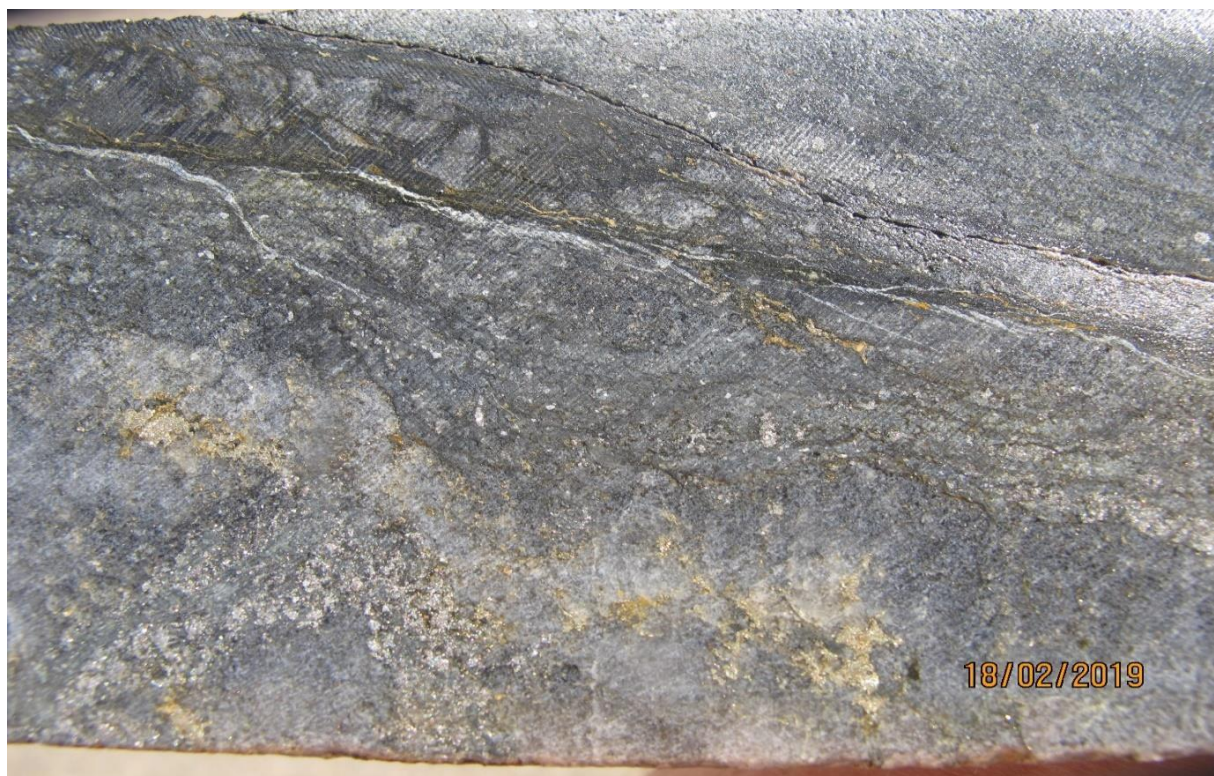
Plate 61: Close-up of quartz veining exhibiting ductile (boudinaged) textures and coarse sulphides.
