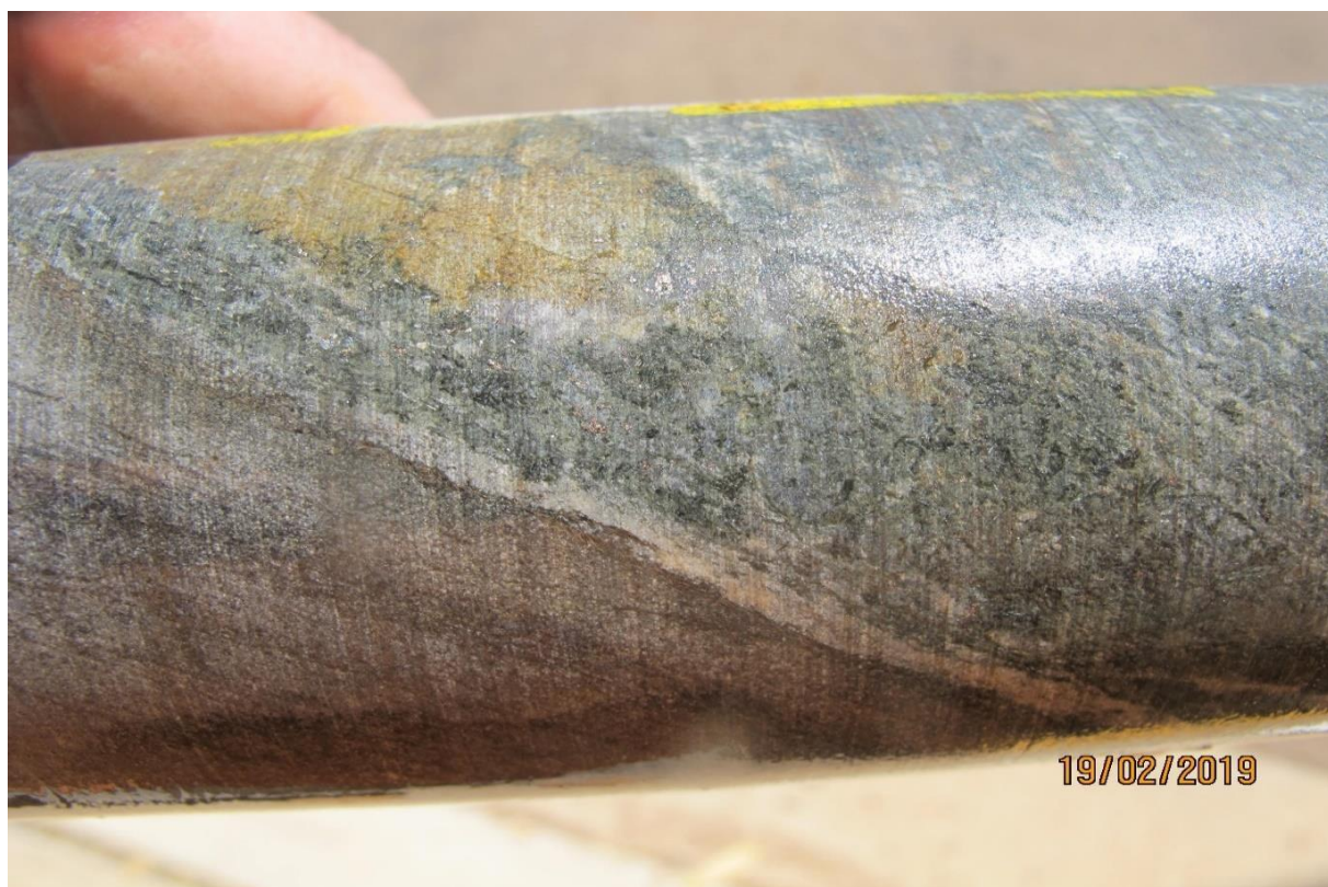
Plate 64: Core interval 73.5 metres depth, showing close-up of lithological variation (interbed) below pale brown garnet-rich horizon.
