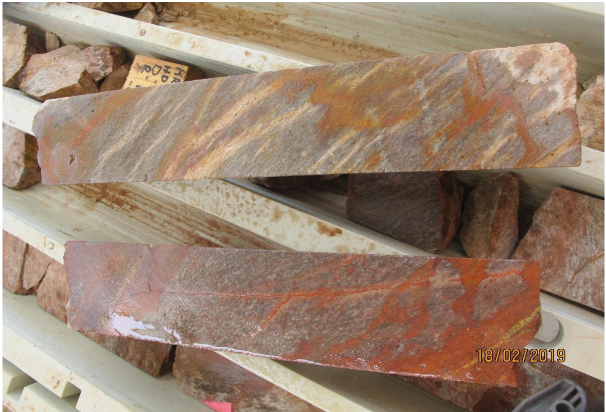
Plate 41: Comparison of core samples above/below 49 metres depth showing increase in silicification and veining. Gold grades ranging from 0.3-0.58g/t Au up to the start of stronger silicification and thin quartz veining at 49 metres depth
