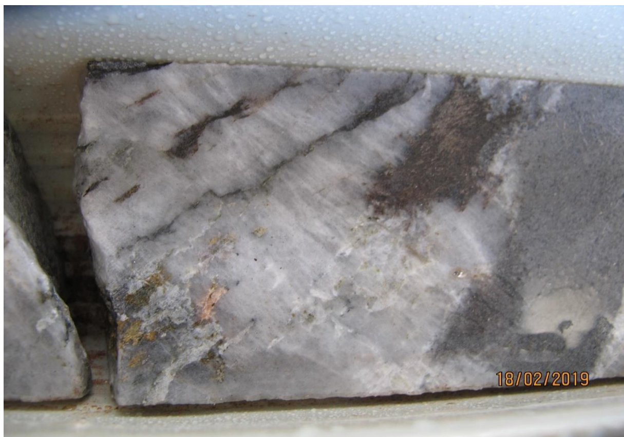
Plate 66: Close-up of cut core sample at 84.1 metres depth, showing coarse quartz veining along with coarse biotite and sulphides; including arsenopyrite, lesser pyrite-chalcocopyrite
