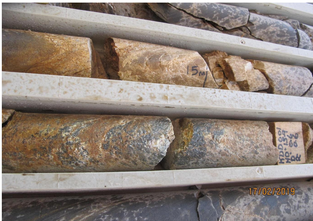
Plate 2: Weakly oxidised calc-silicate unit logged from 14.8 to 16.25 metres.
