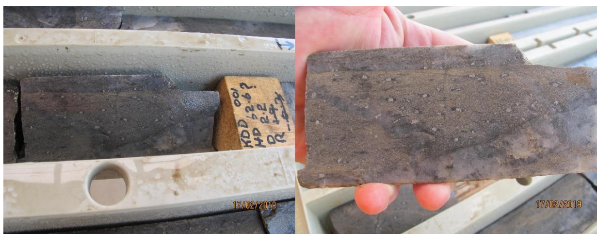
Plates 18 & 19: Core interval 62.5-62.6 metres showing coarse arsenopyrite masses (subhedral to euhedral) which are aligned to the remnant foliation and pre-date cross-cutting quartz veining.
