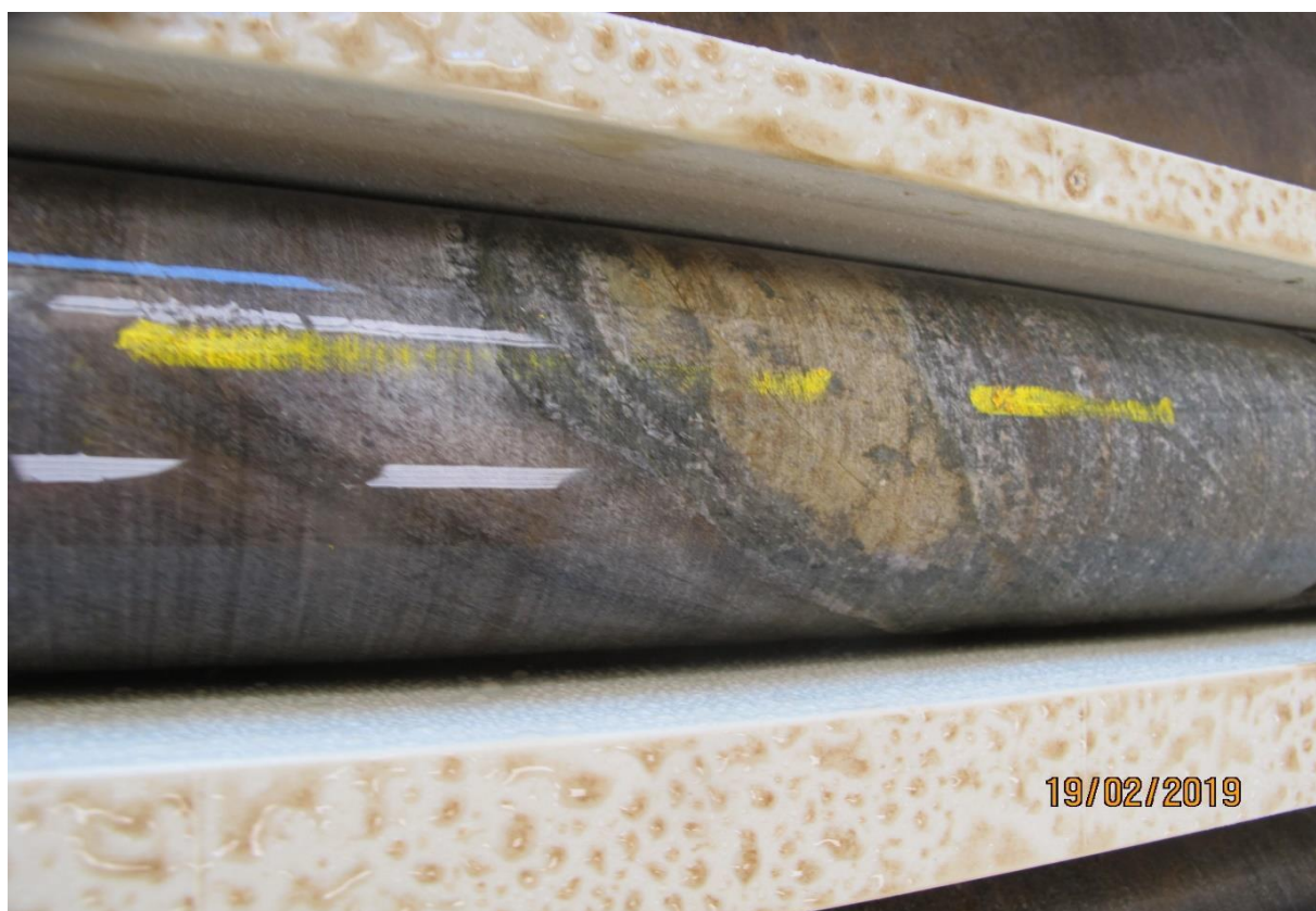
Plate 63: Core interval 73.5 metres depth, showing pale brown garnet-rich horizon which shows ductile deformation.
