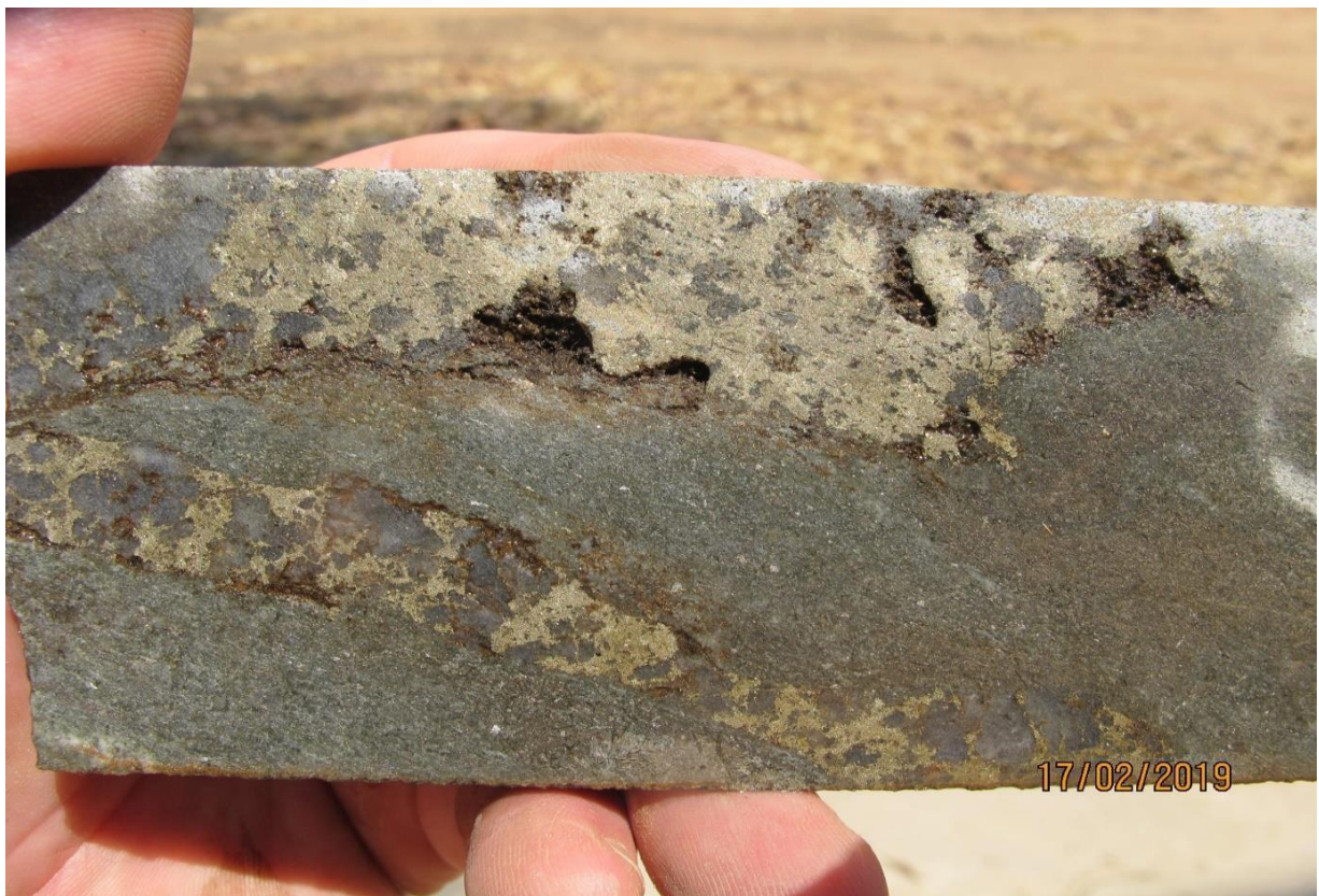
Plate 28: Close-up of core sample 68.2 metres depth showing close to massive pyrite and chalcopyrite infilling within brecciated quartz matrix. Quartz host cross-cuts remnant fabric but appears to be partially constrained by the pre-existing foliation.
