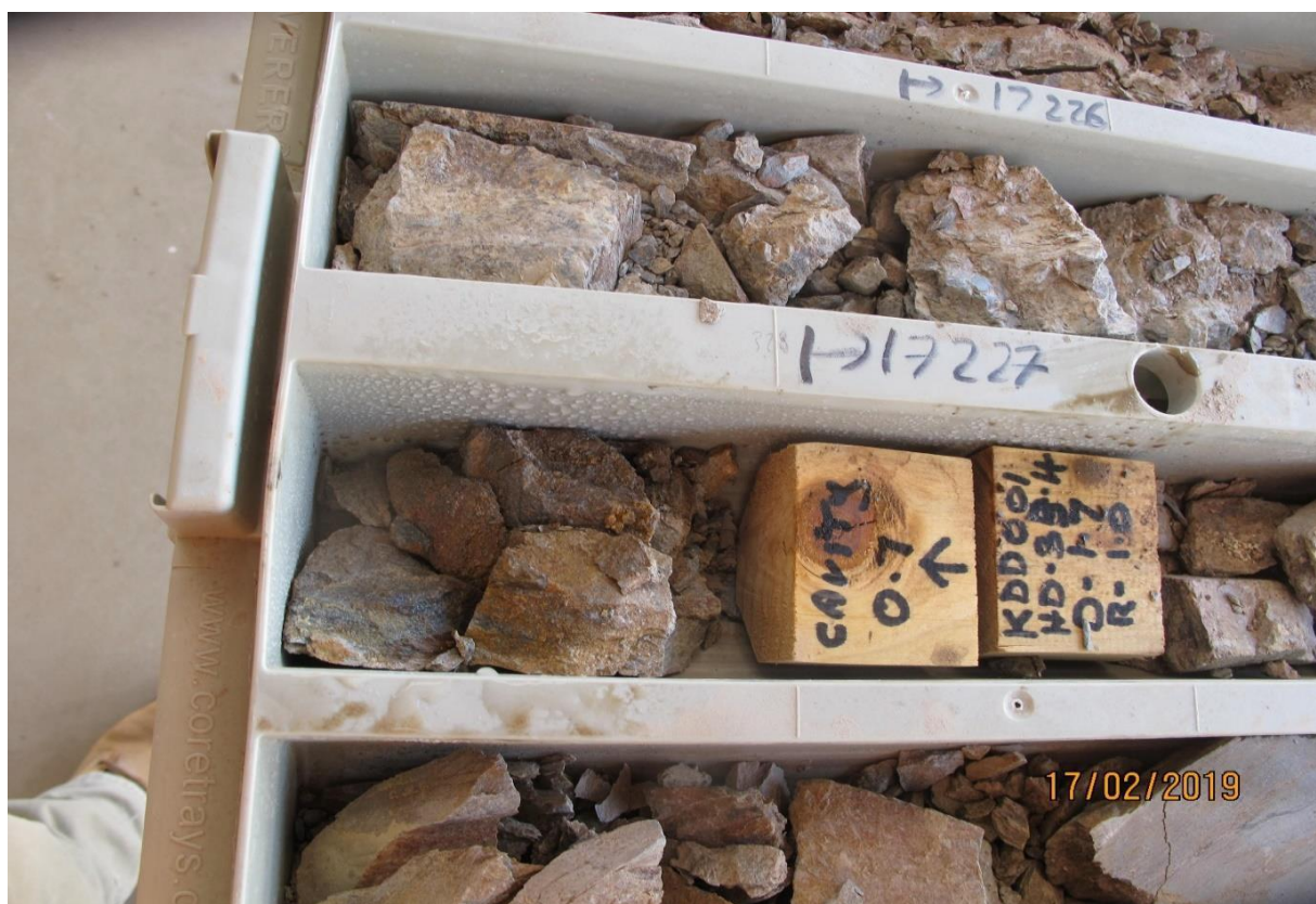
Plate 3: Poor sample recovery from 32.8 to 33.4 metres which may be a small mineralised zone. Assay results may not be representative owing to poor sample recovery.
