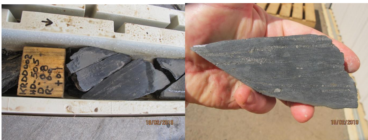
Plate 54 & 55: Core sample from 50.5 metres depth, showing weakly silicified metapsammite. Bands of coarse arsenopyrite appear concordant with the remnant sedimentary-foliation fabric and suggest arsenopyrite genesis was a function of regional metamorphic upgrading prior to the gold emplacement at Kroda-3. This sample is interpreted to be a thin zone of internal dilution within a wider mineralised zone.
