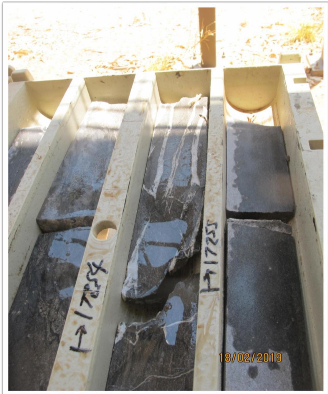
Plate 30: Coarse calcite veins and veinlets logged from 74 metres depth. Veins cross-cut the foliation in a random manner and contain annealing textures.
