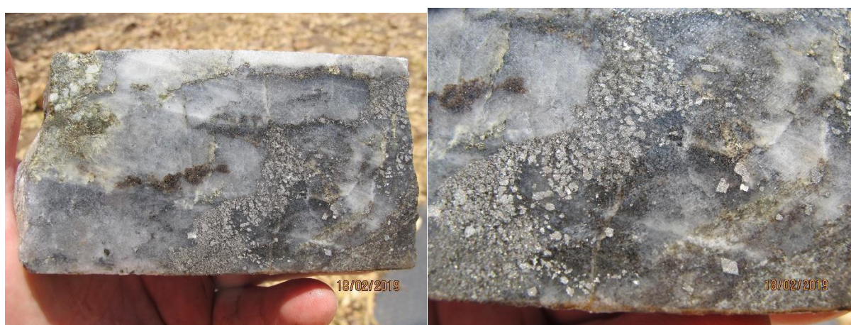
Plates 37 & 38: Core sample from 84.4 metres depth, showing massive quartz veining and coarse sulphide masses. This sample comprised part of the interval which contained the highest gold grades for this sampled zone (1.88 & 1.96g/t Au from 83-85 metres). Gold grade and width of zone suggests that this veining is associated with low-grade footwall mineralisation
