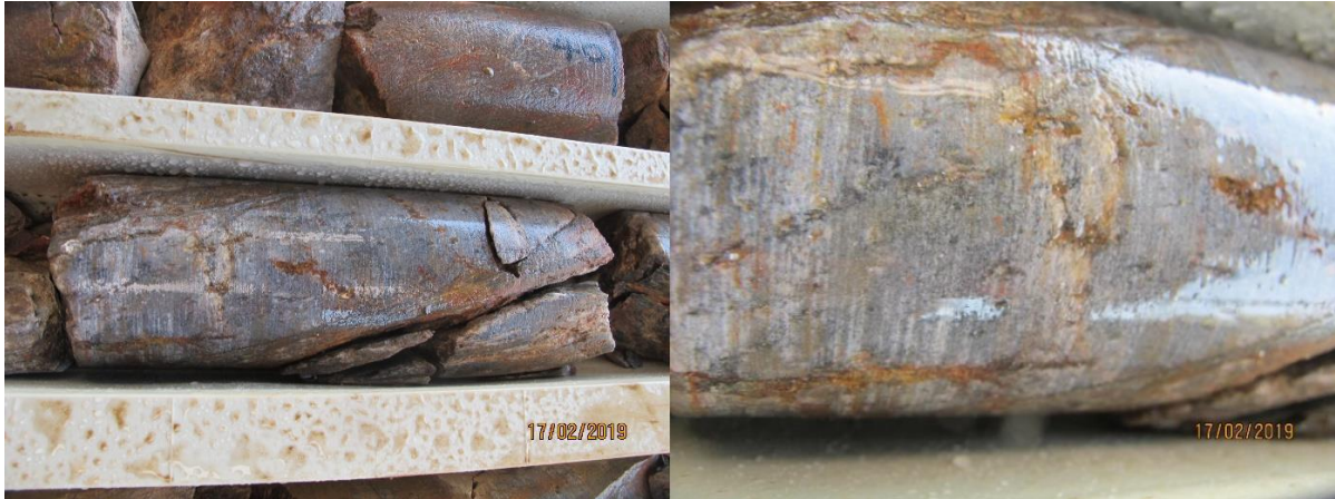
Plates 4&5: Interval 40.6 to 40.8m showing strong silicification and haematite fracture infillings.
