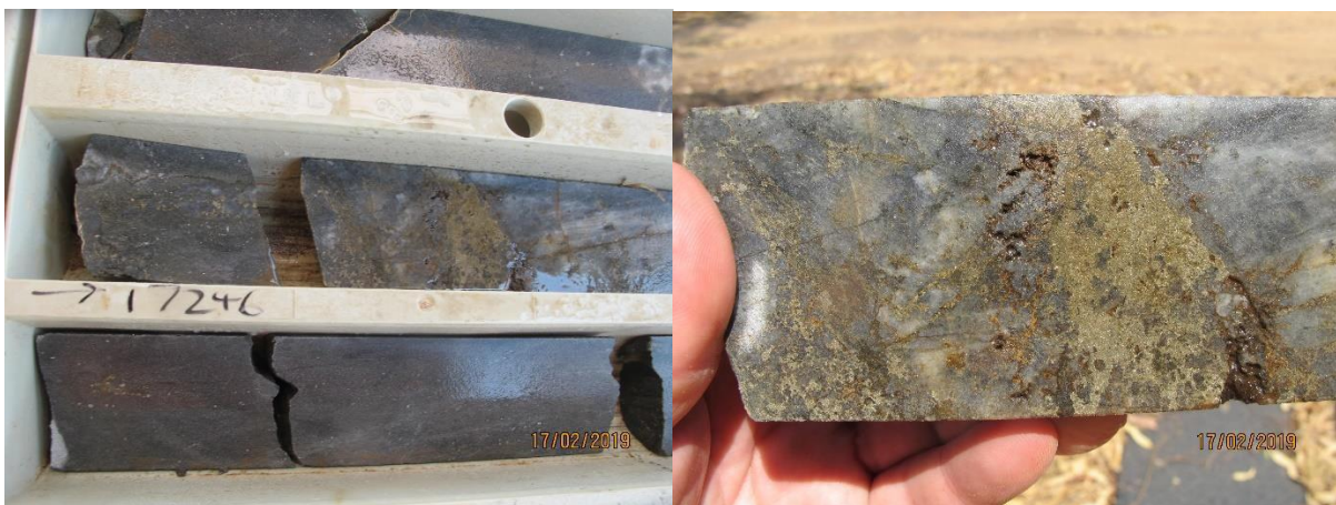
Plates 24 & 25: Core interval 66-67 metres, showing coarse pyrite-chalcocopyrite emplacement within a heavily brecciated massive quartz vein. Sample 17245 was assayed at 9.14g/t Au from 66-67 metres.
