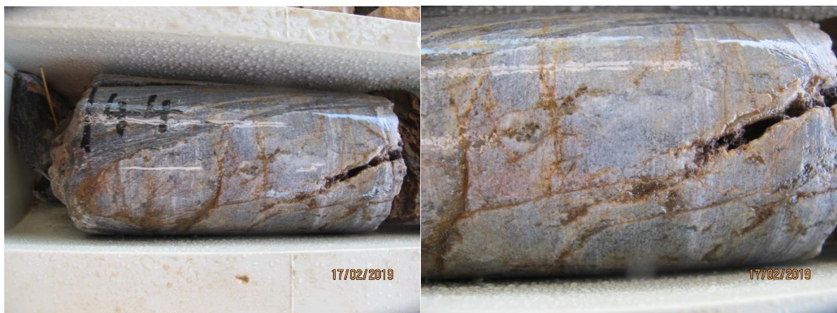
Plates 6&7: Interval 44 to 44.1 metres showing coarse quartz veining, sub-parallel to foliation.
