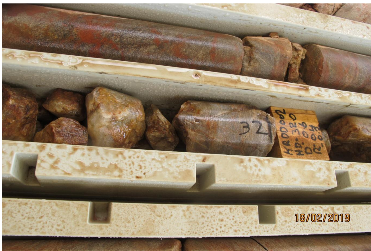
Plate 40: Interval of massive quartz vein logged from 31.5-32.05 metres depth. Broken core with rounded textures suggested drilling intersected a broken zone with significant core loss being identified.
