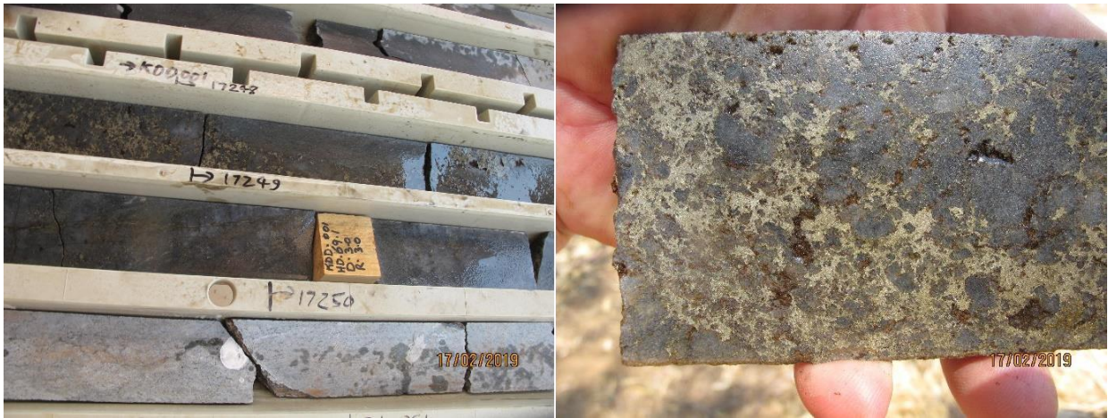
Plates 26 & 27: Core interval 67.8-70.5 metres. Close-up of core sample 67.9 metres depth showing close to massive pyrite and chalcopyrite infilling within brecciated massive quartz matrix.
