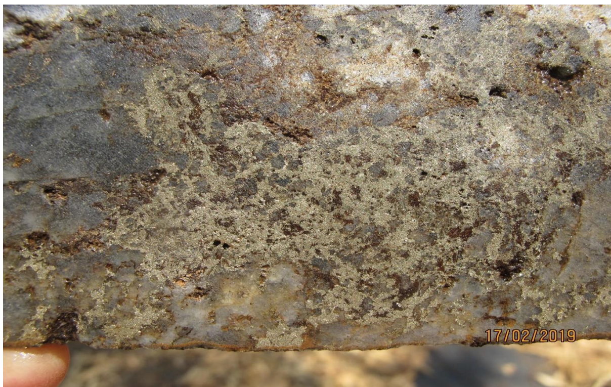
Plate 29: Close-up of core sample 68.4 metres depth showing close to massive pyrite and chalcopyrite infilling within brecciated quartz matrix.
