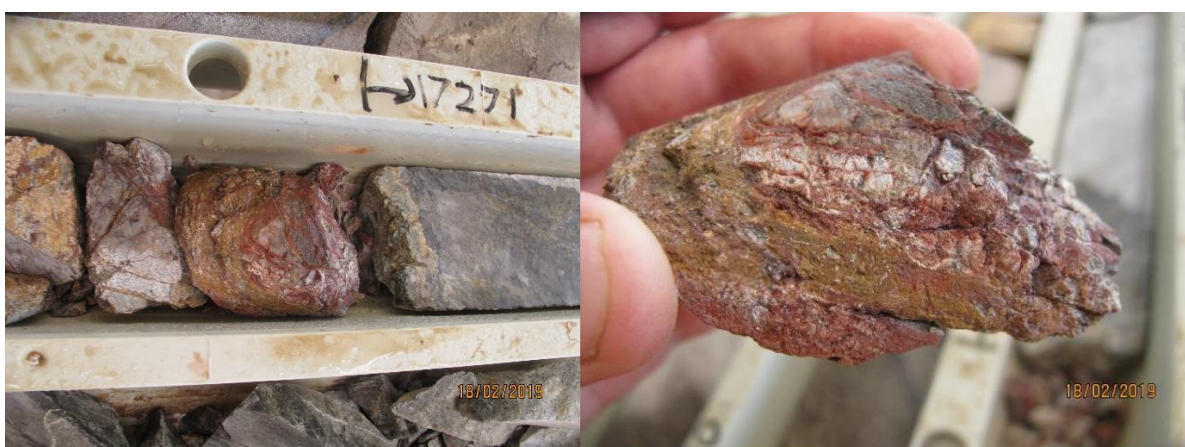
Plates 48 & 49: Core samples 48.9-49.05 metres depth, showing a thin brecciated zone comprising strongly haematitic/brecciated metapsammite with clay infillings above a contact with massive quartz veining at 49.05 metres depth
