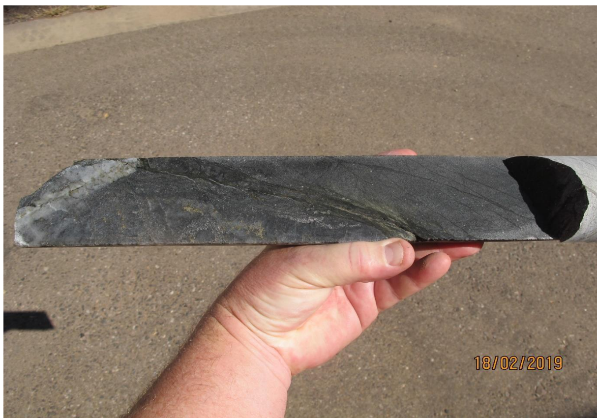
Plate 60: Core interval 53.6-54 metres depth (end of sampled interval. Quartz veining was noted to continue to a depth of 53.95 metres as was indicated in the original geological log which was only 5cm above the end of the sampled interval.
