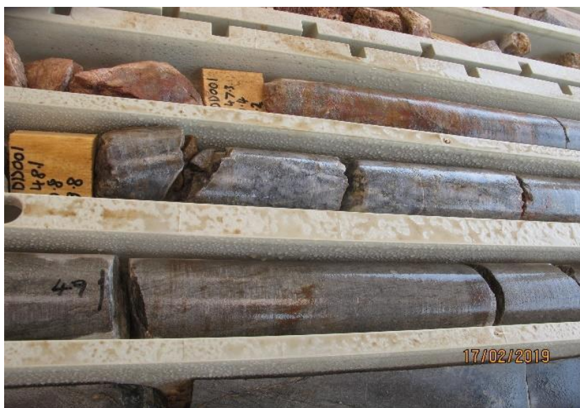
Plate 11: Interval 47.05 to 50 metres was not sampled, but contains heavily silicified metapsammite which has a similar bleached appearance to core that was sampled from 50 metres depth.
