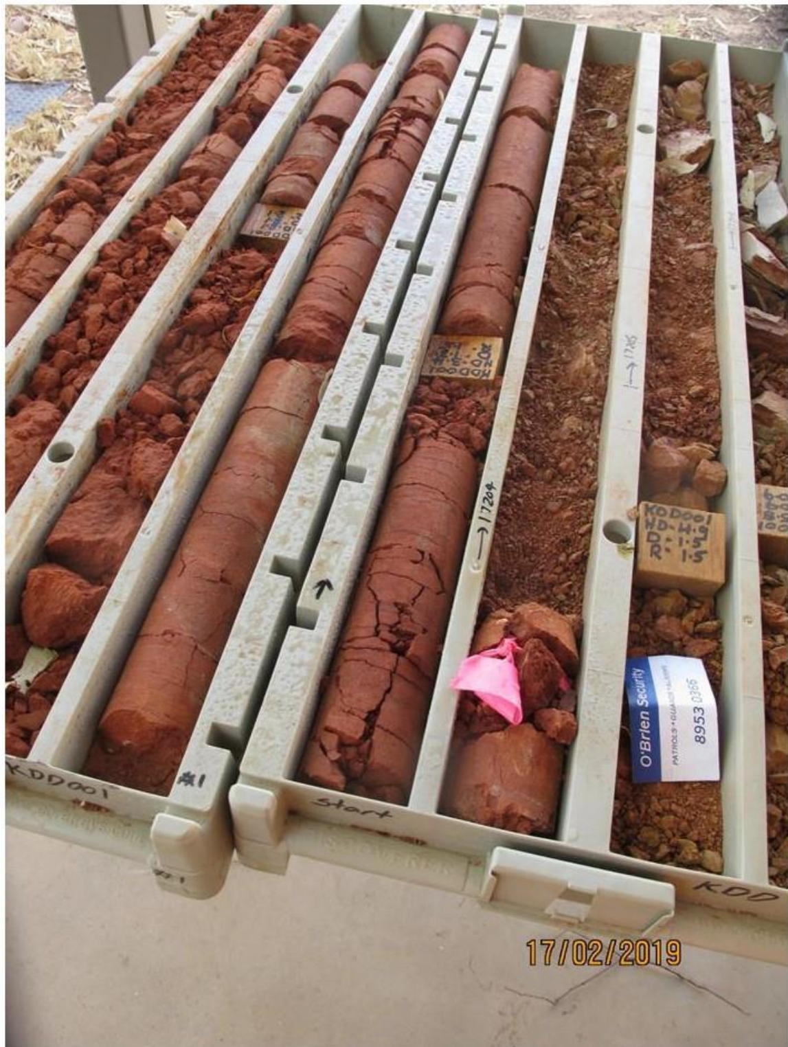
Plate 1: First two core trays for KDD-001, showing transported red-brown sands/clays to the contact with underlying saprock contact at 3.9 metres.
