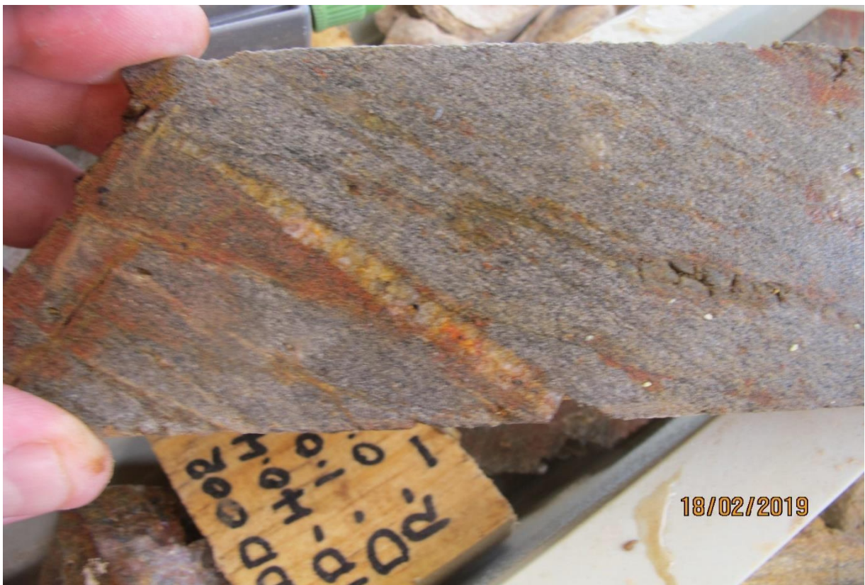
Plate 42: Thin quartz vein with lensoidal symmetry, emplacement concordant to remnant foliation
