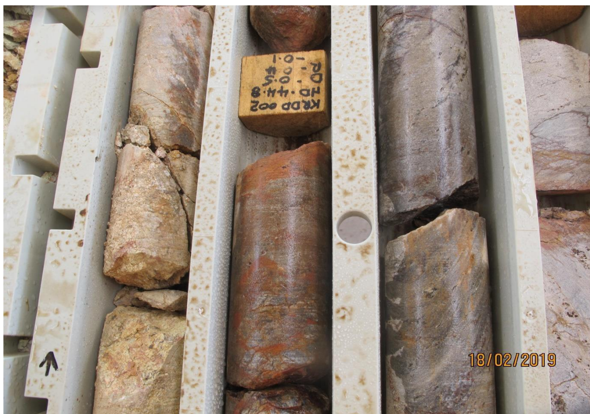
Plate 44: Core interval showing base of calc-silicate unit and silicified and haematite-mottled metapsammite below.
