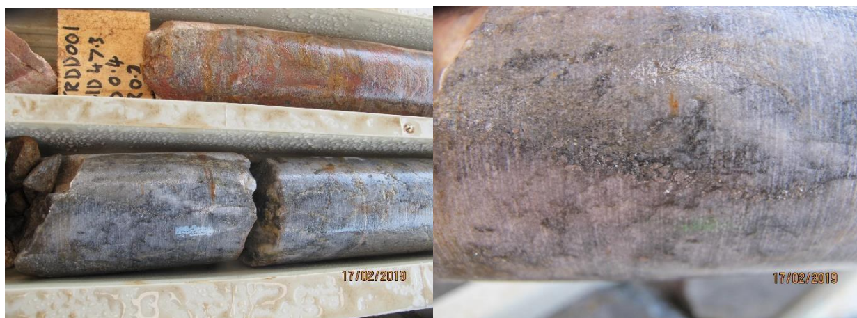
Plates 12 & 13: Interval around 48 metres depth showing strong silicification and coarse sulphides.
