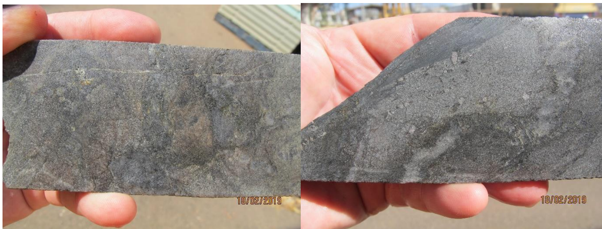
Plate 52 & 53: Core samples from 50.2 metres (left) and 50.7 metres (right), showing degree of variation of textures and alteration within the main mineralised zone for Hole KDD-002.
