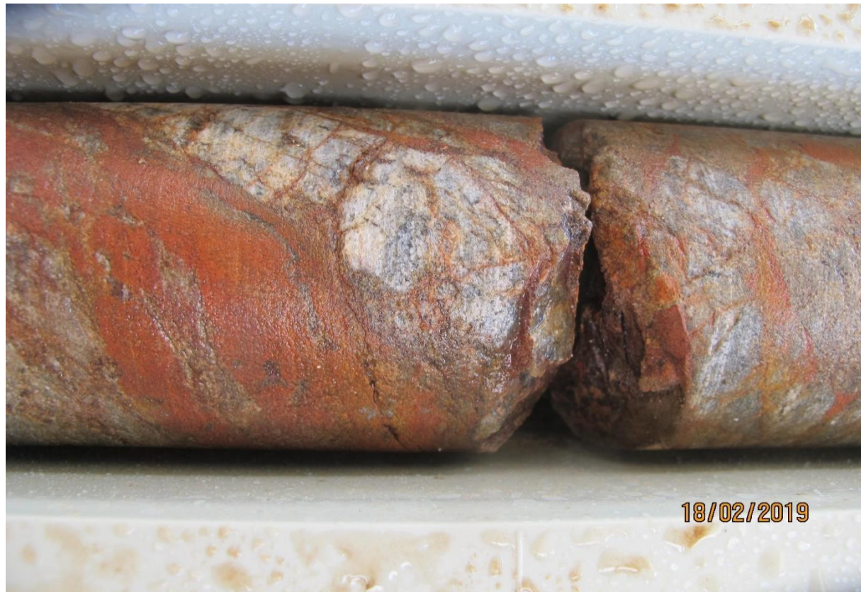
Plate 45: Core sample at 44.9 metres depth, showing quartz veining and strong haematite-mottling.
