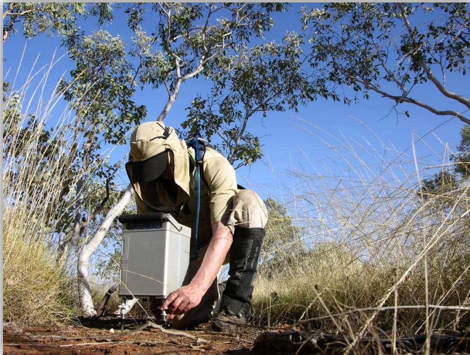
Photo 8 – A Surveyor levelling a Scintrex CG5 gravity meter
