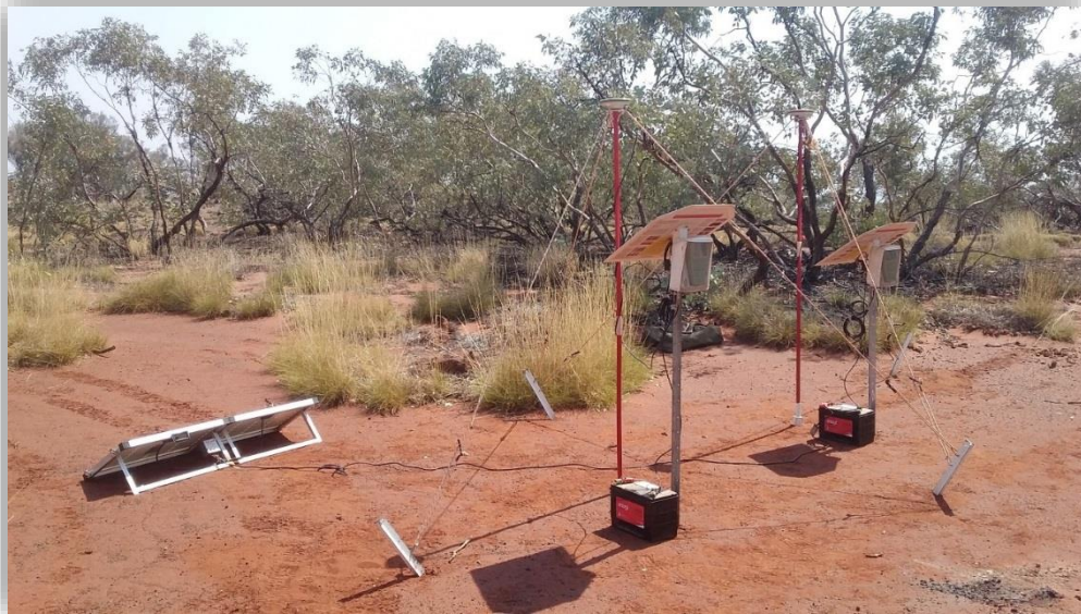
Photo 6 – A Leica GX1230 GNSS receiver set up over base 1537 with a redundant base set up nearby
