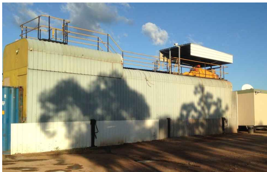
PHOTO 10: Modular Flowsort X-ray Sorter housed in a mobile caravan
