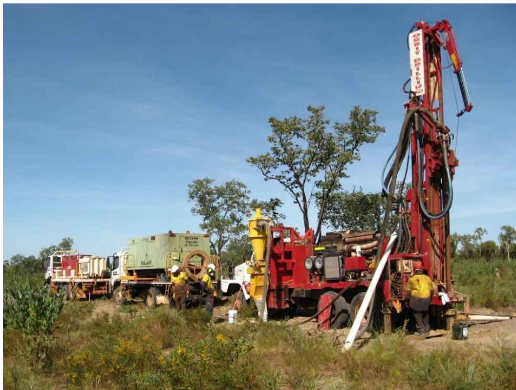
PHOTO 1: Orbit Drilling Hydco RC 40 drill rig with booster compressor
