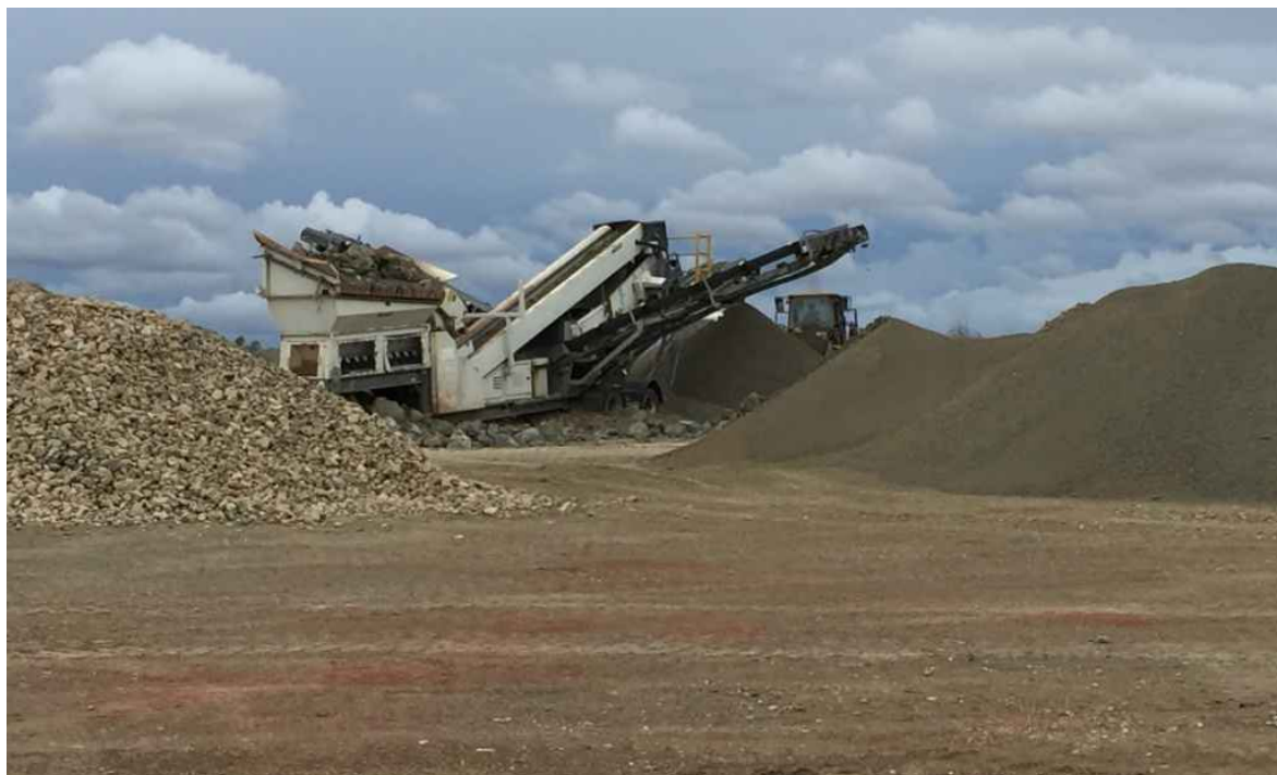
PHOTO 16: Mobile screening plant used to prepare the TOMRA feed into the three size fractions
