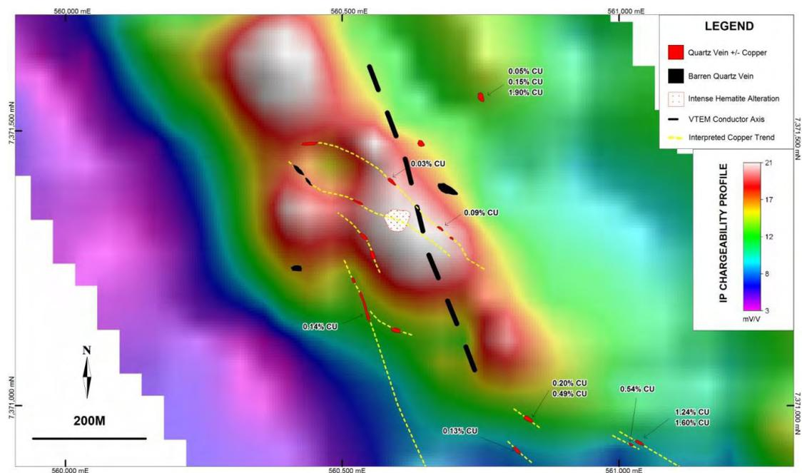
Figure 9: Chargeability anomaly with geological mapping.
