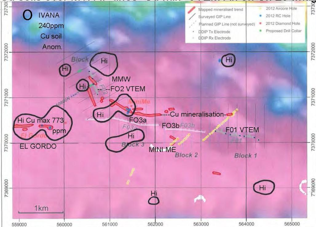
Fig.4c Mini Me IP survey location plan showing outcropping copper mineralisation (red), VTEM
