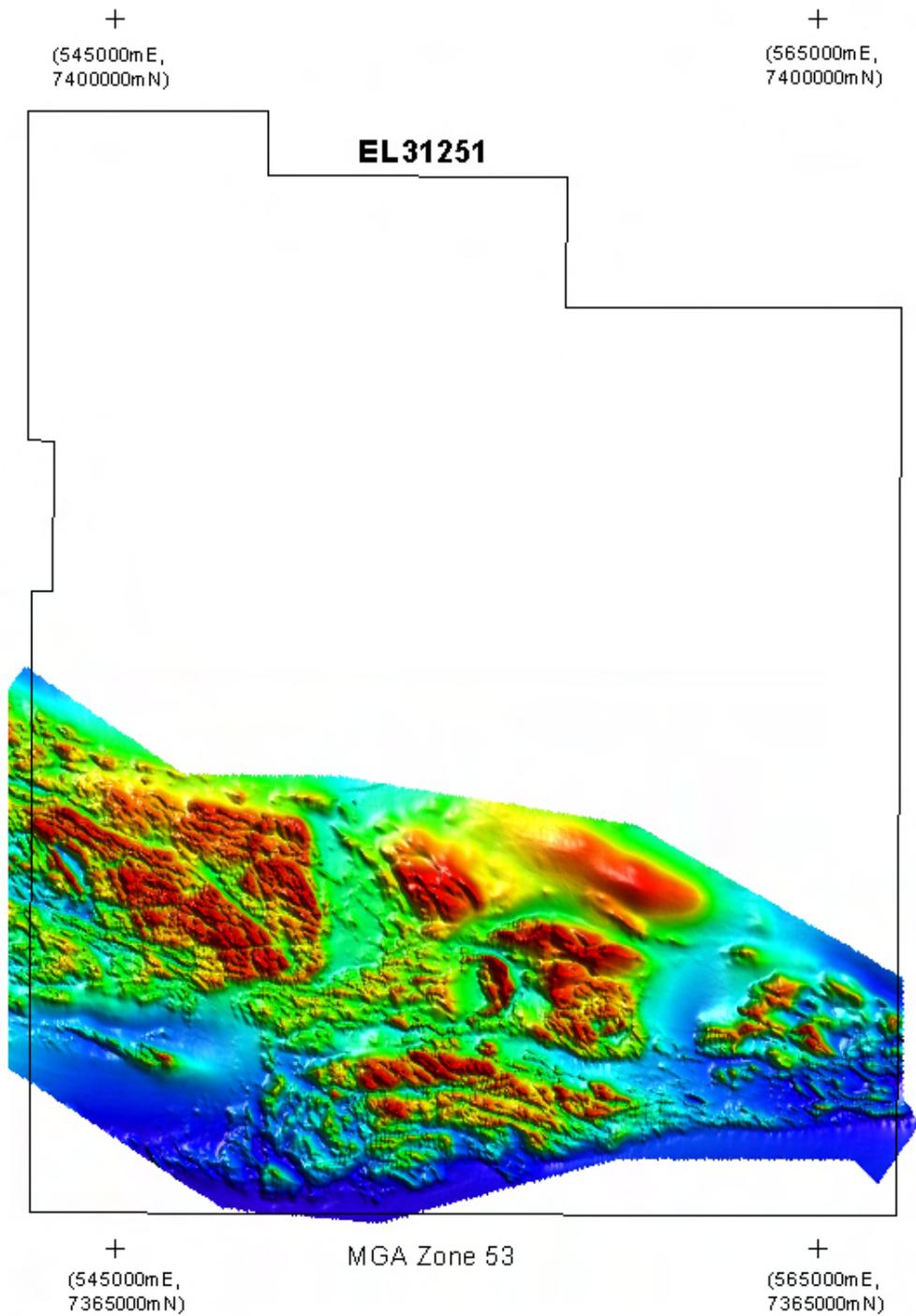
Figure 5a EL31251 Re-processed heli-magnetic survey using 100 meter line spacing flown in 2012. Reduced to the pole magnetics.
