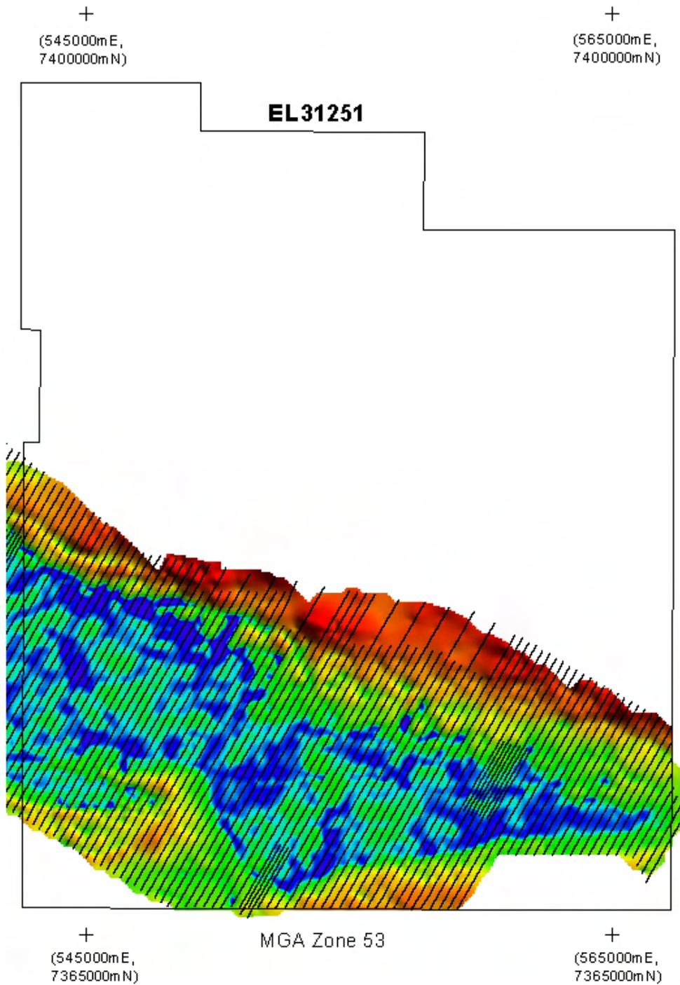
Figure 5g EL31251 Results of AEM depth transformations carried out showing conductivity at 200 meters depth below surface and survey flight lines. (data source for this image dB/dt)
