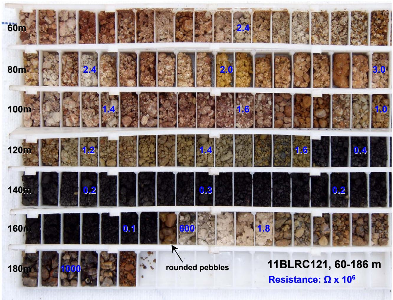
Figure 42. Annotated photograph of the chip trays containing washed cuttings from 60 to 186 m depth in drill hole 11BLRC121. The annotations in blue are apparent electrical resistances of chips (in ohms x 10<sup>6</sup>) measured with a digital multimeter.
