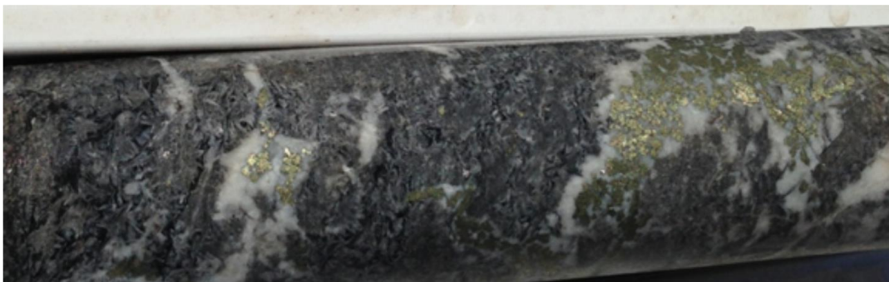
Figure 27: Core from CCD02 (Pacifico diamond hole drilled 2015) – 146m, chalcopyrite (no pyrite) mineralisation in ex- evaporite bed packed with bladed gypsum pseudomorphs.
