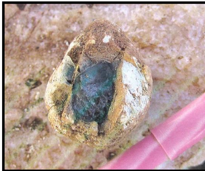
Figure 5.1: Example of uranite porphyroblast/concretion from PNC's Trench 4 at Yambla (UXA Structural Geology Report CR2011-1170). Note clay alteration/radiation damage surrounding crystal.
