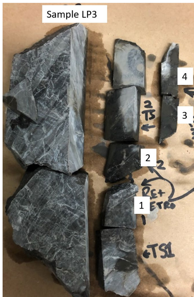
Fig. 1. Photograph of sample LP3 sent to USGS for HP experiments, showing the rock fragments analyzed for TOC content and pyrolysis properties (labeled 1-4, see also Table 1).
