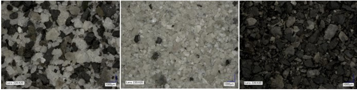
Figure 28 - Moroak Sandstone from Beetaloo W-1 at depths of 2010-2013 mMDRT (left), 2073-2076 mMDRT (centre), and 2175-2178 mMDRT (right)
