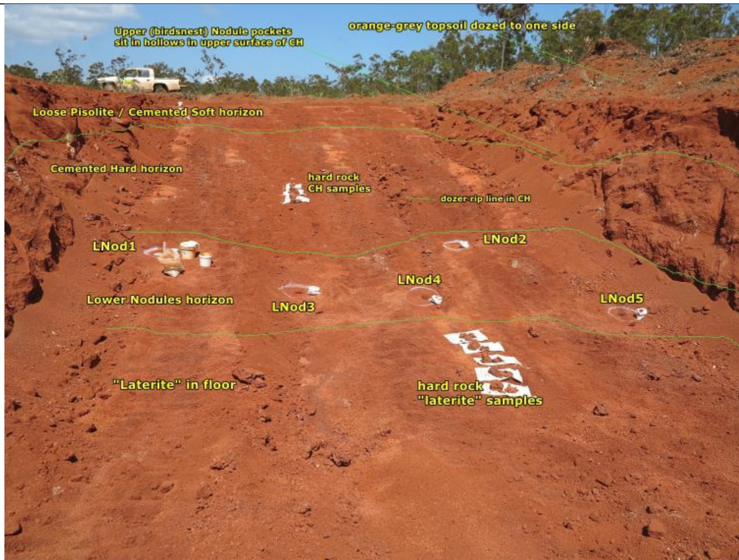
Figure 7 Geology and "soft" sampling locations in density pit 15GDP-05 ("West")
