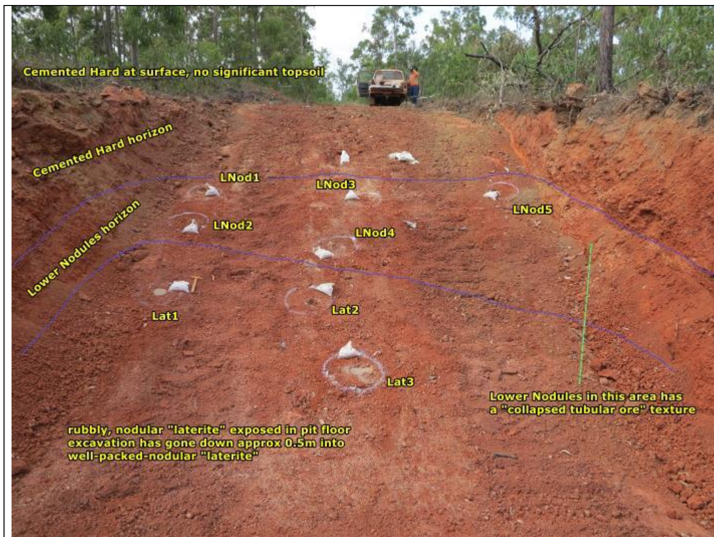
Figure 12 Geology and "soft" sampling locations in density pit 15GDP-10 ("Southeast Tree-rats")
