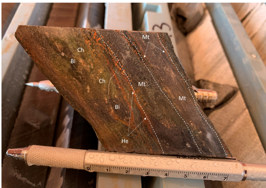
Figure 10. Localised alteration, showing Biotite (Bi) to chlorite (Ch) and magnetite (Mt) to hematite (He).
