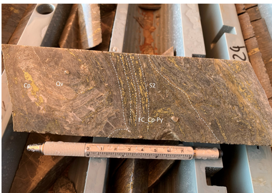
Figure 12. Post S2 deformational quartz vein (Qv) with chalcopyrite (Cp) and foliation-controlled (S2) chalcopyrite and pyrite mineralisation (FC_Cp-Py).
