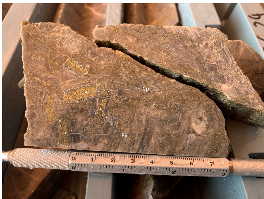
Figure 14. Post deformational brecciated quartz vein. Pyrite (Py) chalcopyrite (Cp). Porphyroclasts containing chalcopyrite and pyrite.
