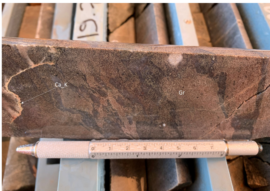
Figure 9. Quartz vein with localised micro garnet (Gr) alteration, with a thin diffuse carbonate-feldspar (Ca-K) veinlet.
