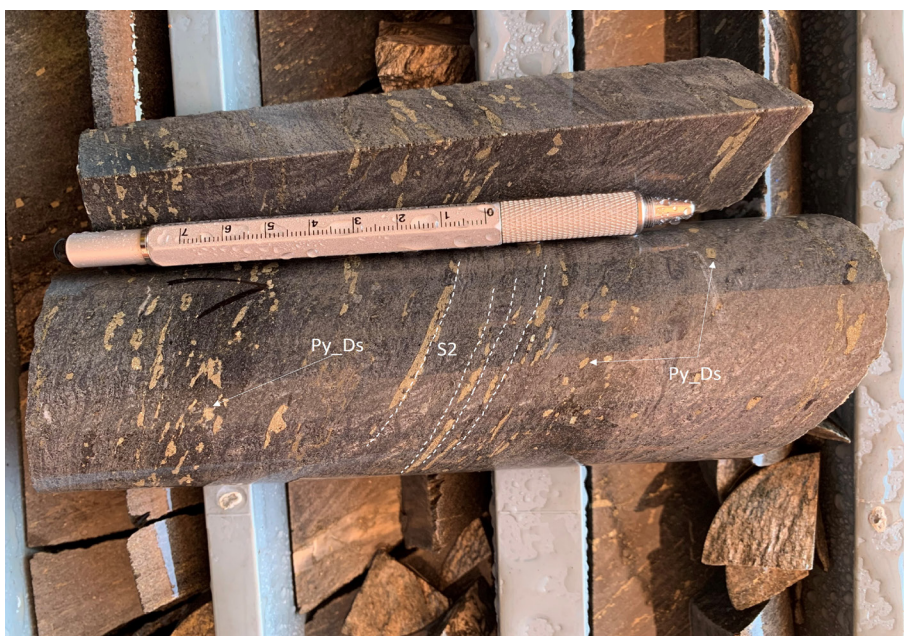
Figure 11. Disseminated pyrite (Py_DS) and (S2) foliation-controlled pyrite.
