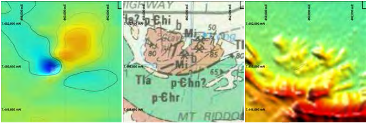
Figure 13: A. The TMI grid and the anomaly in dark blue, and the modelled body outlined faintly in black; B. An excerpt from the 1:250k Geological map (Shaw and Wells, 1983), showing the position of faults, mica mines and different lithologies Ehi = Iridina Gniess, Ehn = Calcareous member of Iridina Gniess, Ehr = Riddoch Amphibolite. C. STRM topographic grid.
