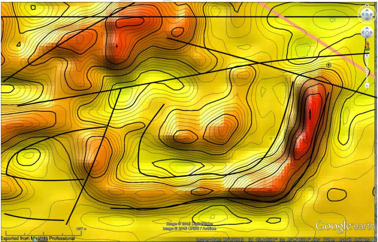
Figure 5: The ASO_RTP transformation of the TMI highlights a “U-shaped” anomaly just south of the tenement.
