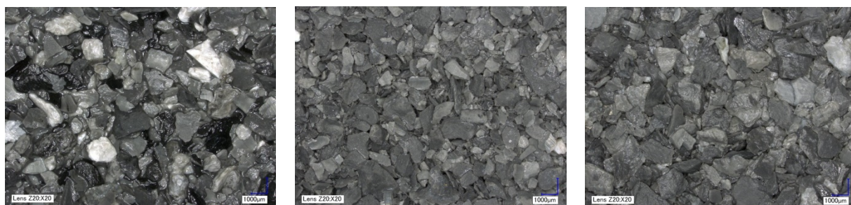
Figure 21 – Lower Velkerri cuttings in Kalala S-1 well at 2571-2574 mMDRT (left), 2592-2595 mMDRT (centre) and 2616-2619 mMDRT (right).
