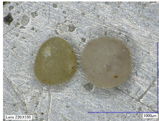
Figure 14 - Hole fill from 407 mMDRT indicative of positive penetration of the Bukalara Sandstone
