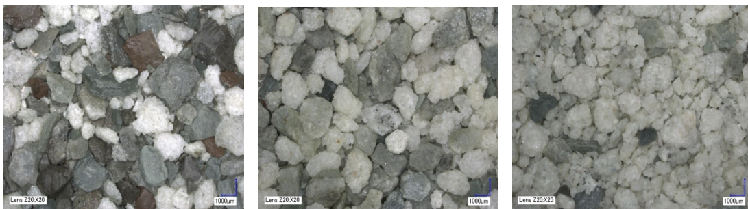
Figure 16 – Bukalorkmi Sandstone in Kalala S-1 well at 845-850 mMDRT (left), 870-875 mMDRT (centre) and 890-895 mMDRT (right)
