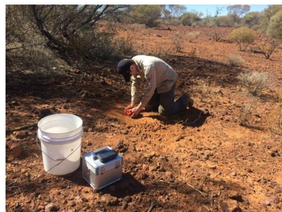
Miniaturised Tromino® seismometer set up for a single passive seismic HVSR station recording for 20 minutes
