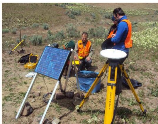
1 seismometer station set up as part of a passive seismic array survey recording for hours Image reproduced from Earth.boisestate.edu
