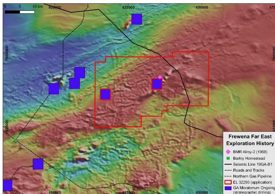
Figure 6 **ABOVE:** TMI map of Frewena Far East displaying location of BMR drill hole Alroy-2 and Ga and NTGS's seismic line 19GA-B1. The two portions blue portions excised from EL 32293 represent areas where stratigraphic drilling is planned by GA and NTGS during 2020
