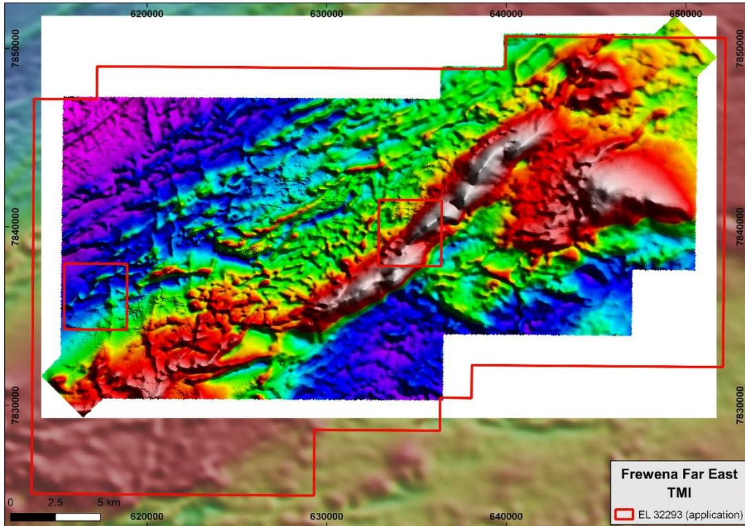
Figure 34 ABOVE: Total magnetic intensity image derived from the detailed AMAGRAD survey over Frewena Far East
