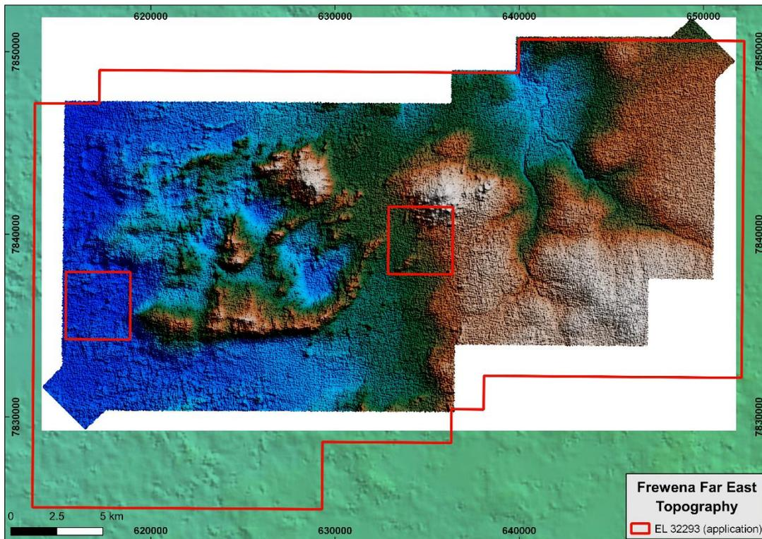
Figure 32 ABOVE: Digital elevation model derived from the detailed AMAGRAD survey over Frewena Far East
