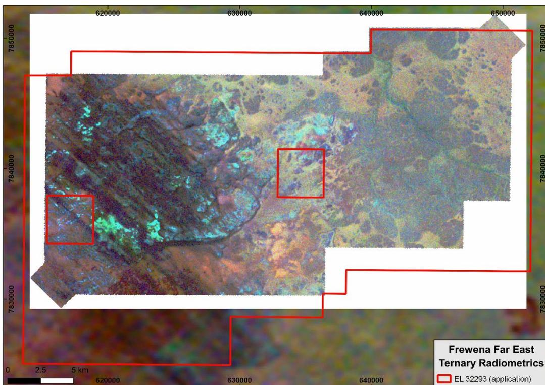
Figure 33 ABOVE: Ternary radiometric image derived from the detailed AMAGRAD survey over Frewena Far East
