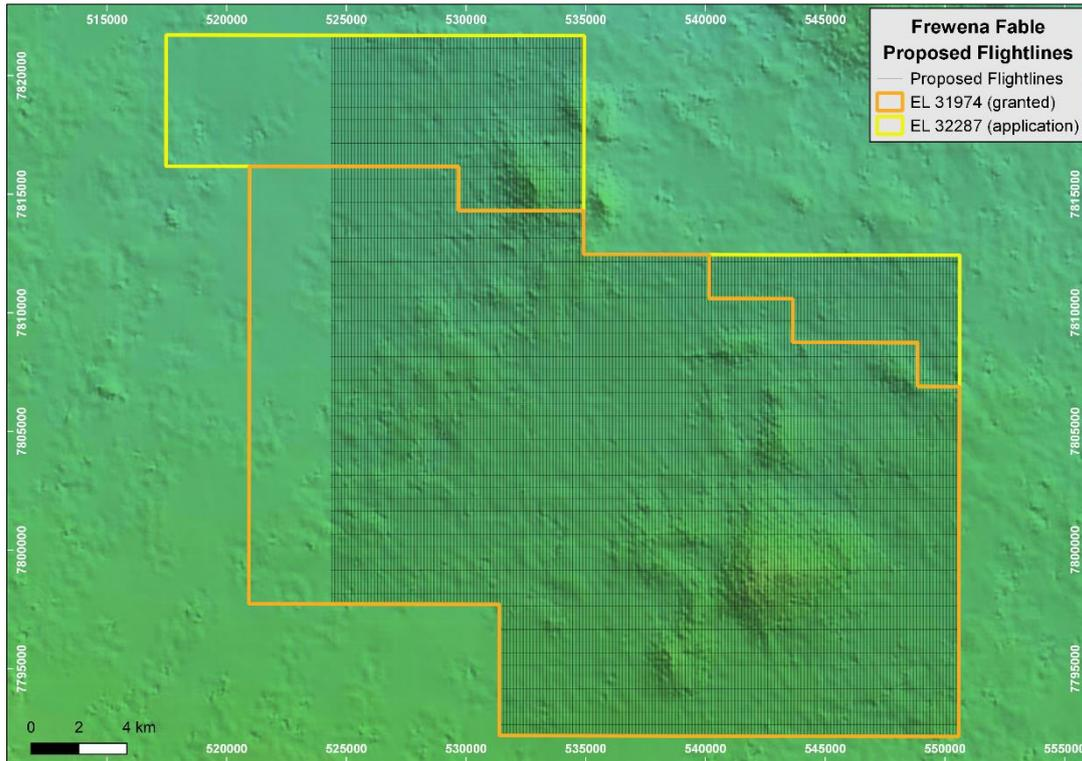
Figure 26 **ABOVE:** AMAGRAD survey flightlines over the Frewena Fable Project were orientated north-south at 50m spacing with east-west tie lines at 500m spacing
