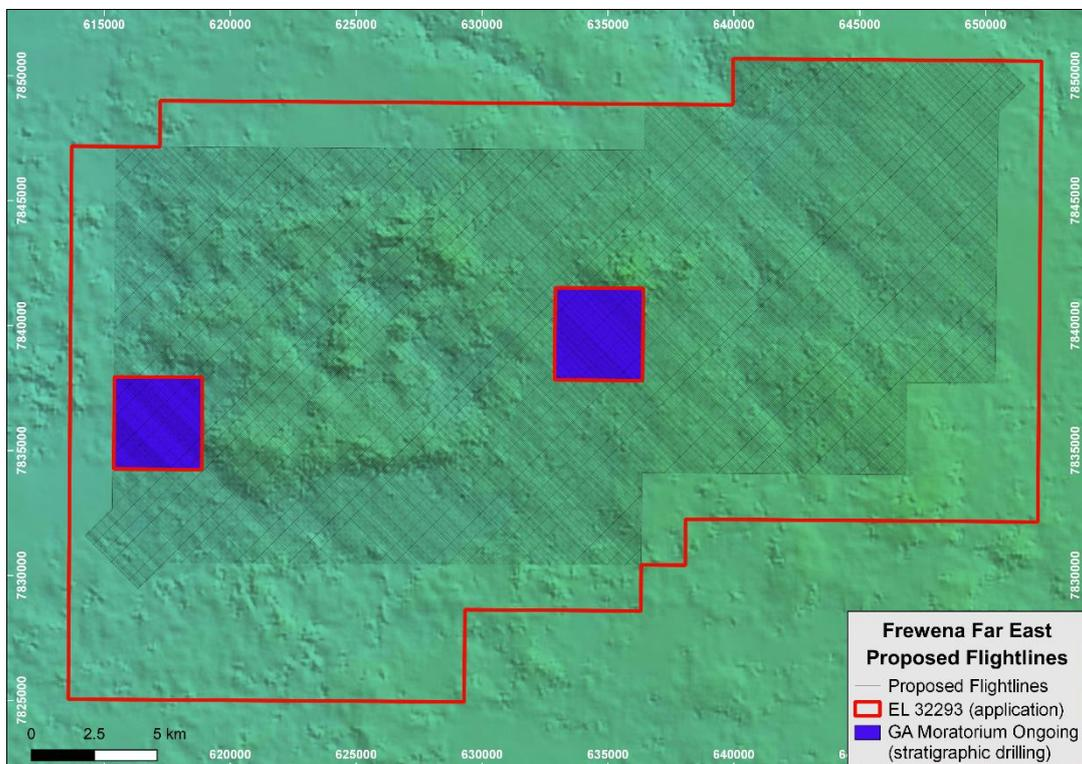
Figure 27 **ABOVE:** AMAGRAD survey flightlines over the Frewena Far East Project were orientated south east – north west at 50m spacing with north east – south west tie lines at 500m spacing; the survey was extended over the two areas excised from EL 32293 where GA and the NTGS have undertaken stratigraphic drilling
