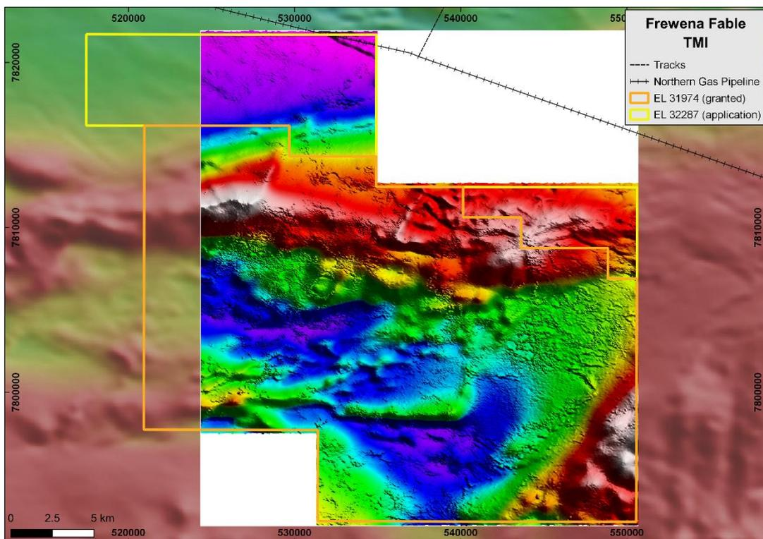
Figure 30 **ABOVE**: Total magnetic intensity image derived from the detailed AMAGRAD survey over Frewena Fable
