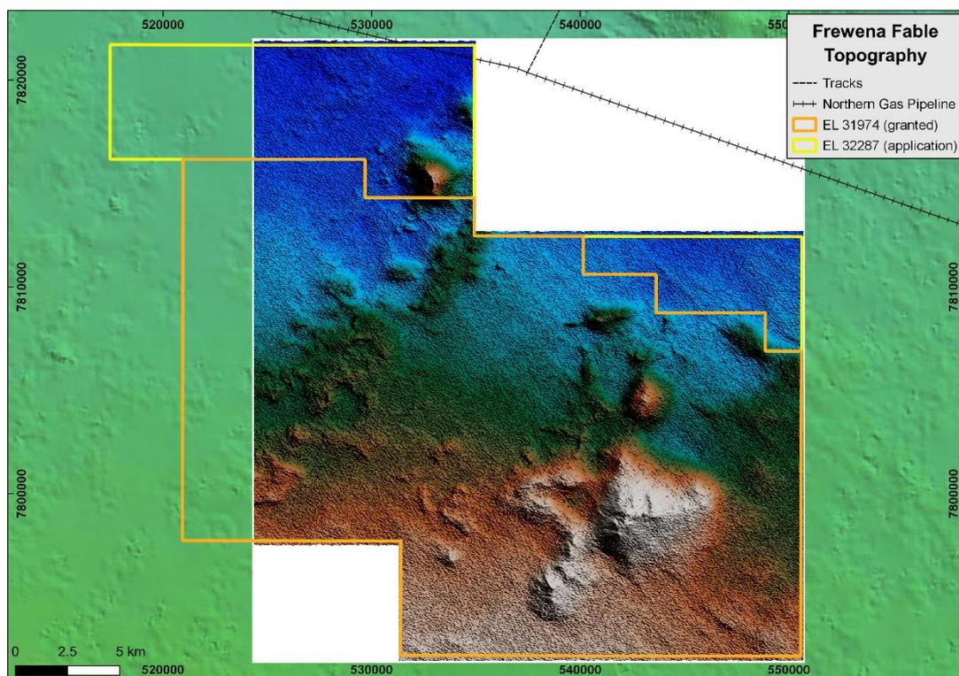
Figure 28 **ABOVE**: Digital elevation model derived from the detailed AMAGRAD survey over Frewena Fable
