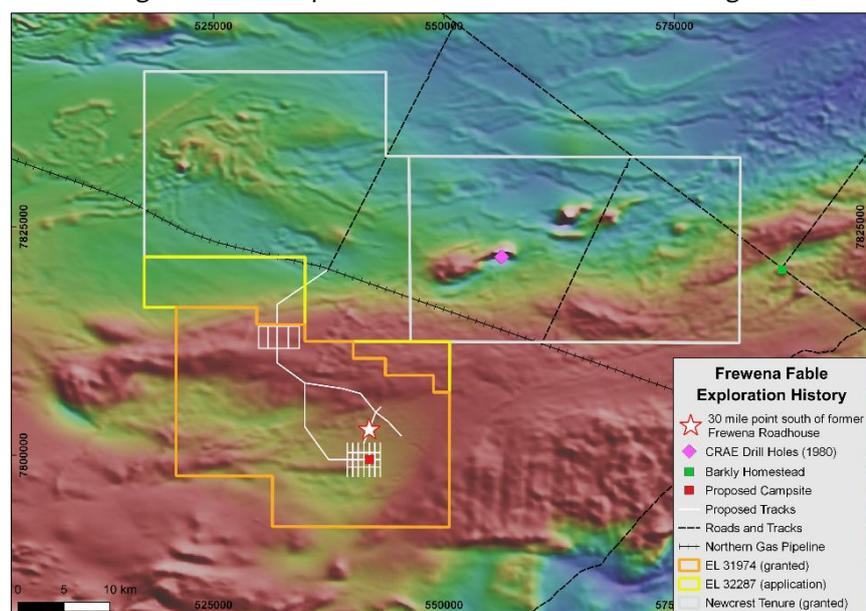
Figure 5 **RIGHT**: Total Magnetic Intensity (TMI) map of Frewena Fable displaying location of the CRAE 1980 drilling north east of the Project and Inca's proposed access tracks under the Company's recently approved MMP
