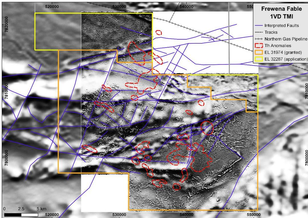
Figure 31 **ABOVE**: 1<sup>st</sup> vertical derivative TMI image derived from the detailed AMAGRAD survey over Frewena Fable
