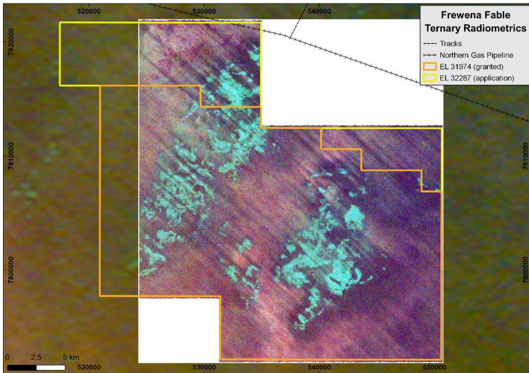
Figure 29 **ABOVE**: Ternary radiometric image derived from the detailed AMAGRAD survey over Frewena Fable
