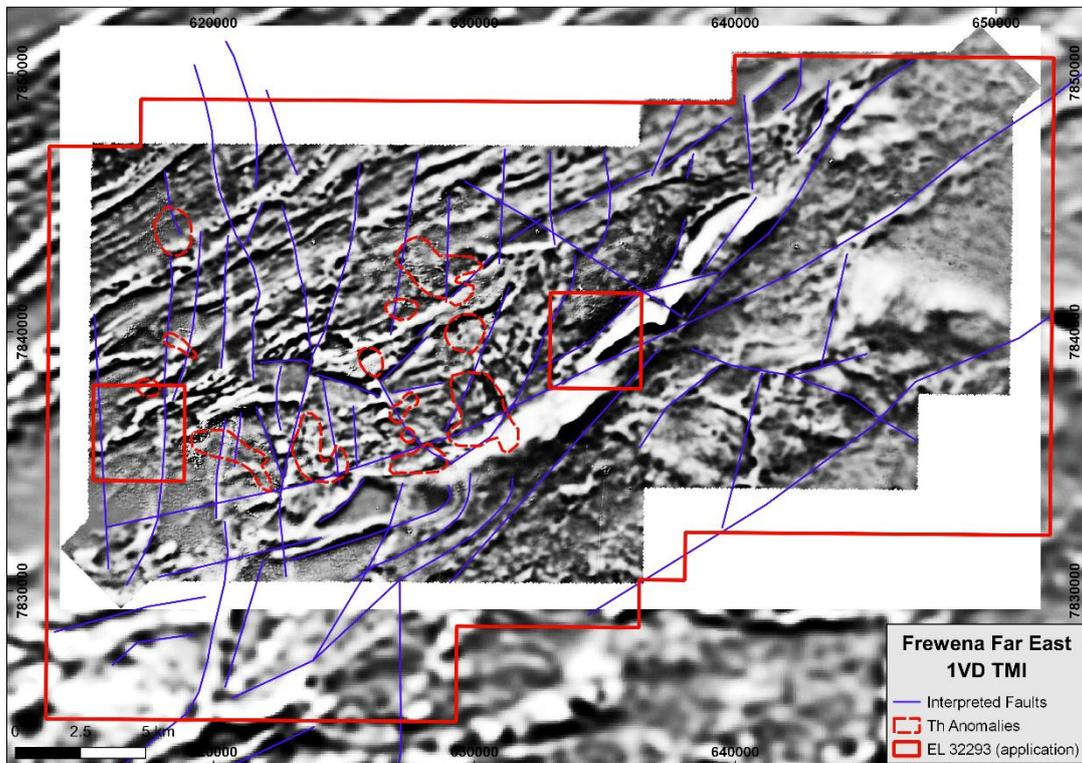
Figure 35 ABOVE: 1<sup>st</sup> vertical derivative TMI image derived from the detailed AMAGRAD survey over Frewena Far East
