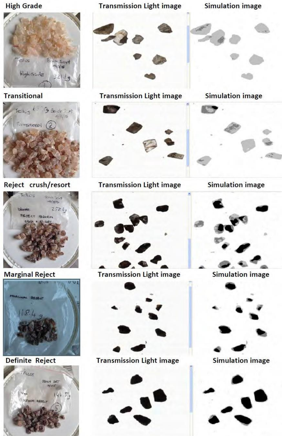
Figure 10: Tellus salt sample classes, transmission light and simulated sorting images
