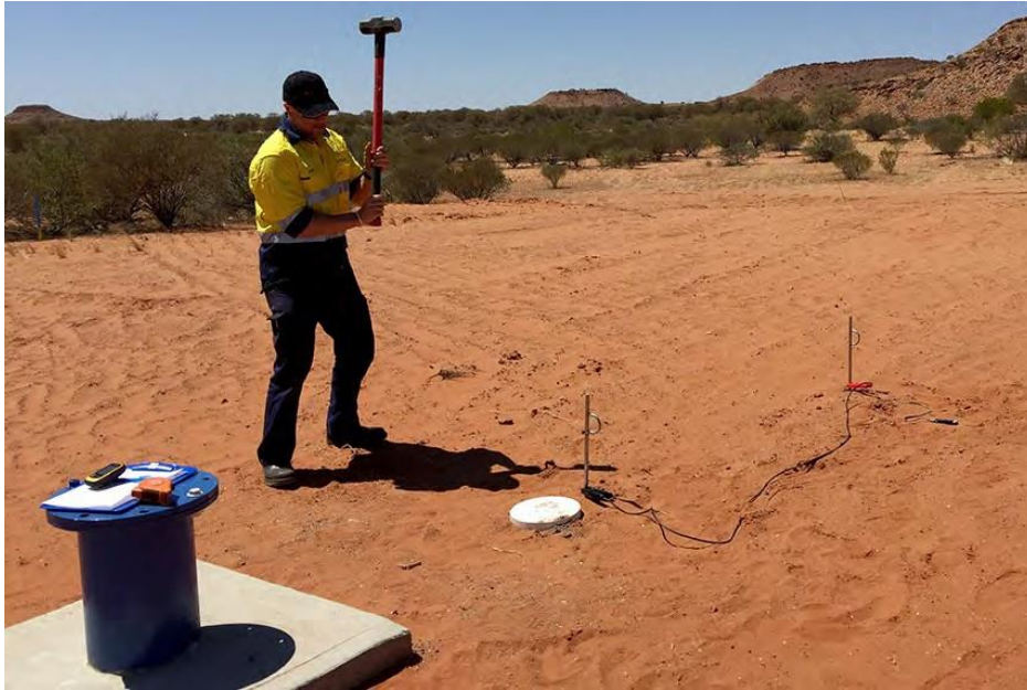
Figure 8: Electro seismic survey at Chandler project site
