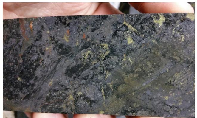
**Figure 5.** Garnet–magnetite rock from Johnnies Reward with chalcopyrite-bearing veins that overprint magnetite. Core is 63.5 mm wide.
