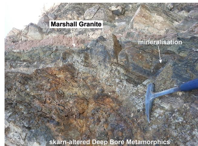
**Figure 4.** Marshall Granite dyke intruding layered and foliated calc-silicate rock of the Deep Bore Metamorphics and producing minor magnetite–scheelite–molybdenite mineralisation below the contact zone at Molyhil. Hammer is 30 cm long.
