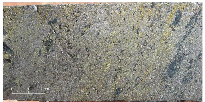
**Figure 3.** Garnet-bearing orthogneiss containing chalcopyrite and sphalerite, with minor pyrrhotite and galena and trace pyrite from Home of Bullion. Core is 63.5 mm wide.
