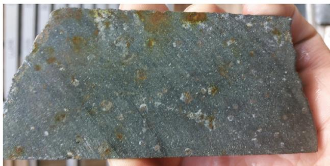
**Figure 2.** Disseminated sulfide assemblage of violarite–chalcopyrite–pentlandite overprinting altered metagabbro from Prospect D. Core is 63.5 mm wide.
