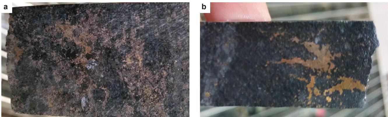
**Figure 6.** Core photos from Oonagalabi. (a) Chalcopyrite, pyrite, and pyrrhotite in garnet-rich zones associated with recrystallised quartz veins in a metamafic rock. Core is 63.5 mm wide. (b) Disseminated veinlets and interstitial sulfides, including sphalerite, pyrite, pyrrhotite, and chalcopyrite within a diopside-rich zone. Core is 32 mm wide.
