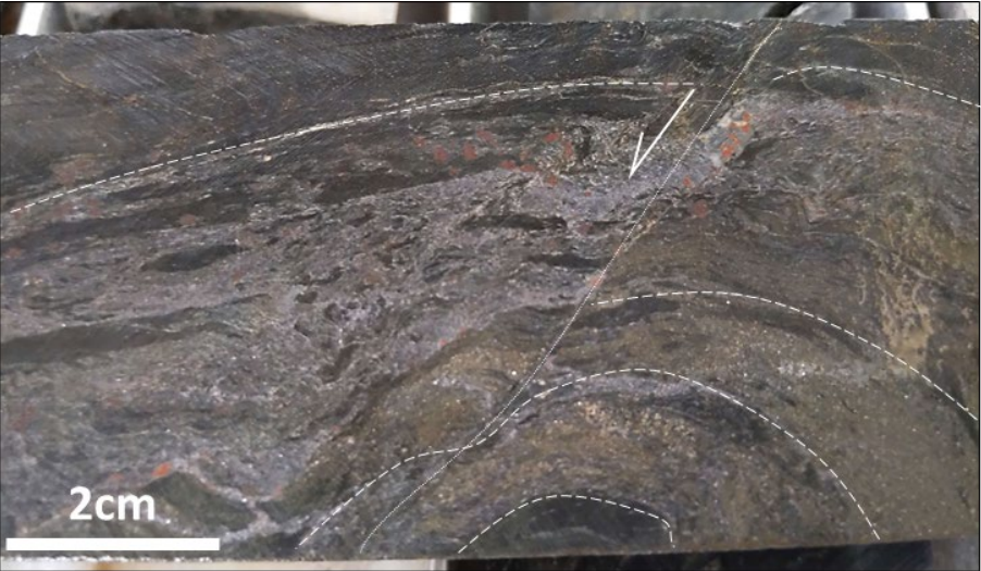
Folded massive to semi-massive sulfides (py-cpy-sph-gn + cb-mt-chl-tlc gangue)
