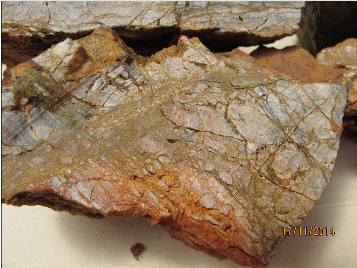
Plate 1: Outcrop sample NJRK_2014_001, consisting of fractures (brecciated) and veined quartz. Sample collected in surveyed area north of Max's Find (423890mE, 7570920mN)
