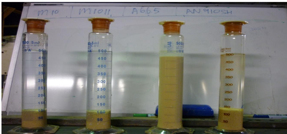
Picture 2: 500ml static cylinder test – APH Tailings
