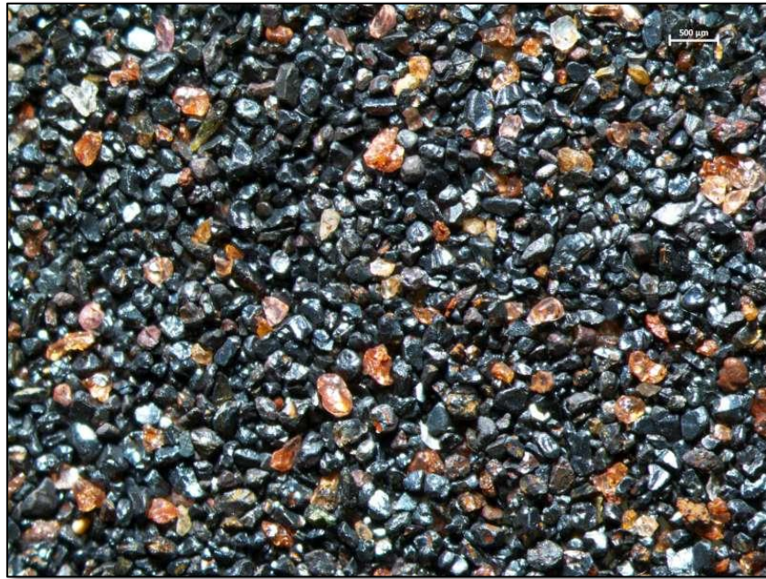
Figure 4 – -250μm + 150 μm Conductor 1 Ilmenite Concentrate.
