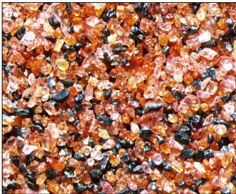
Figure 5 – -250µm + 150 µm final Garnet concentrate.
