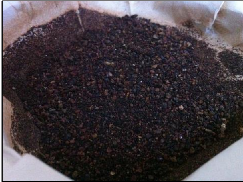
Figure 2 – -2mm + 150 µm HLS Sinks (HM Concentrate) Fraction wet.
