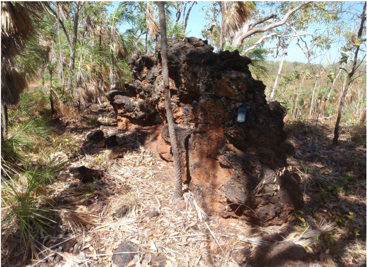
Photograph 4 Goethite-dominant siltstone breccia at Lewis. This material is typical of the mineralisation in the area.
