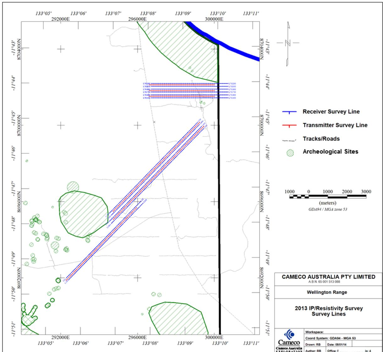
Figure 6: IP/resistivity survey lines.
