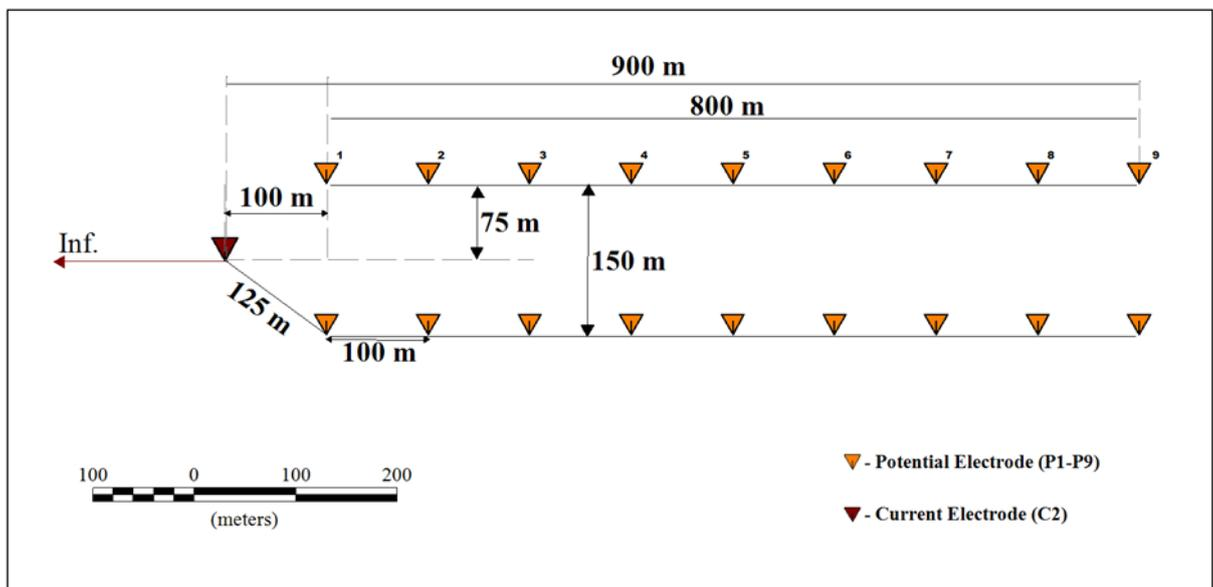
Figure 5: IP/resistivity array layout.
