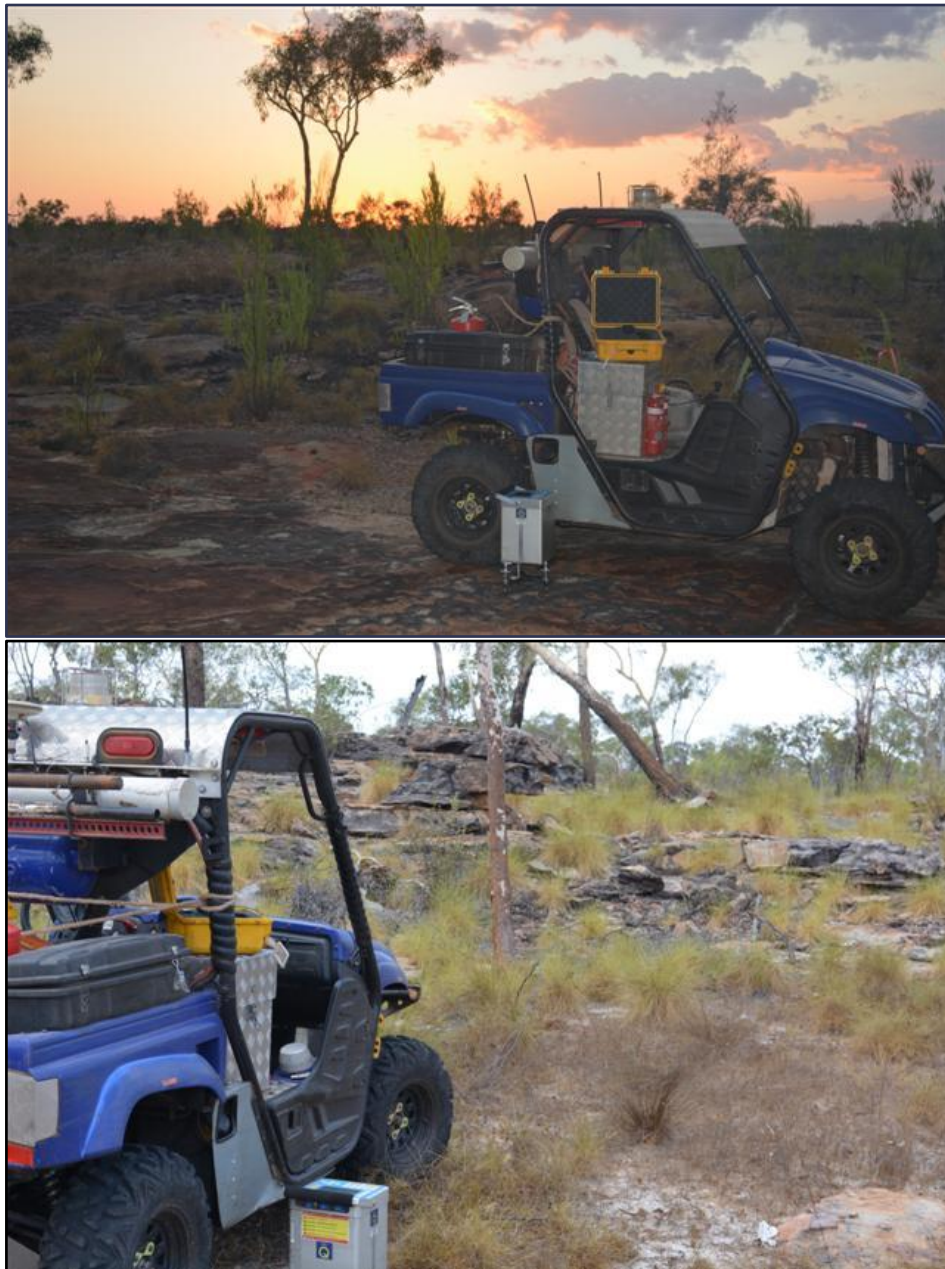
Photos 1-2 – Heavily customised Daishsat ATV (DATV) used for gravity acquisition
