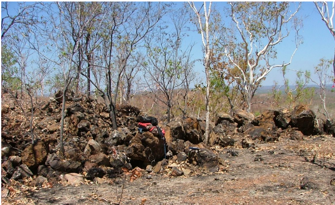
Figure 34: Hewson “ore sorting stockpile” next to pit. The stockpile contains abundant large blocks of siliceous breccia with quartz vein and metasediment fragments, along with gossan infill and occasional sulphide boxworks. Sample 645904 returned: 0.18% Sn, 0.18% As, 634 ppm Pb, 115 ppm Sb, 25 ppm Bi, 132 ppm Cu, 2.2 ppm Ag, & 0.06 ppm Au (with low Zn).
