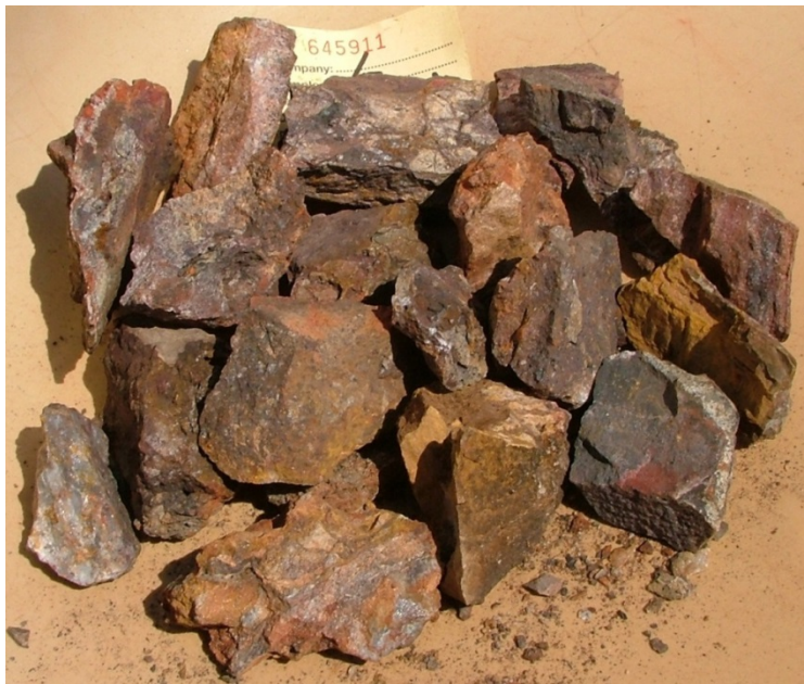
Figure 31: Example chips of sample 645911 located within the altered zone south of Mavis. This float (sub-outcrop) sample of altered and veined metasediment returned: 0.80 g/t Au, 1120 ppm As, 105 ppm Bi, 254 ppm Cu & 85 ppm Pb, (with low Ag, Zn, Sb & Sn).
