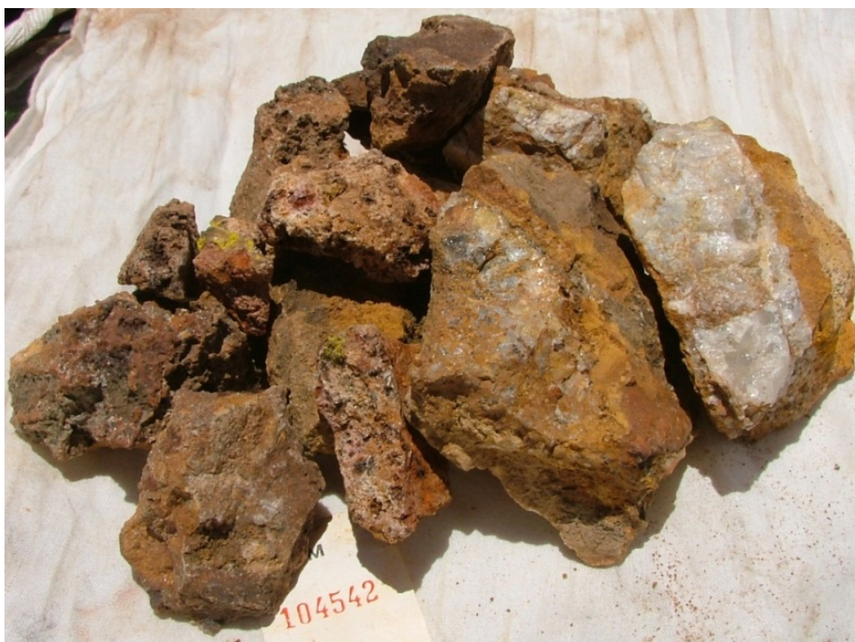
Figure 21: Example chips from sample 104542 that came from a 5-10m wide fluidised breccia pipe on Jason's Peak. The breccia is strongly altered and cut by later quartz veining. The sample returned assays of 0.55% Pb, 0.47% As, 0.24% Sb, 0.15% Bi, 211 ppm Sn, 26.6 ppm Ag, & 0.09 ppm Au (with low Cu & Zn). Given the high lead assay, it is probable the abundant yellow-brown "limonite" is partly plumbo-jarosite. There may also be some scorodite (arsenic oxide) present.
