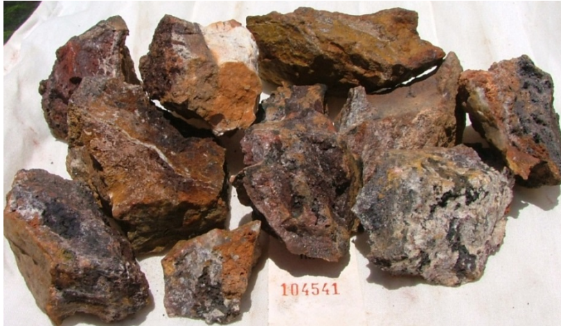
Figure 30: Example chips from sample 104541 located within the centre of the auriferous alteration-vein zone about 200m south of the Mavis mine. The sample is from a 3-4m wide Quartz-Gossan-Vein zone with sub-parallel quartz veins in altered metasediment (Mount Bonnie Formation?) with FeOx as disseminations, patches and filling voids. Analysis returned a high gold value of 1.25 g/t Au, along with 716 ppm As, 38 ppm Bi, & 138 ppm Cu. Results for Ag, Pb, Zn, Sb & Sn were all low.
