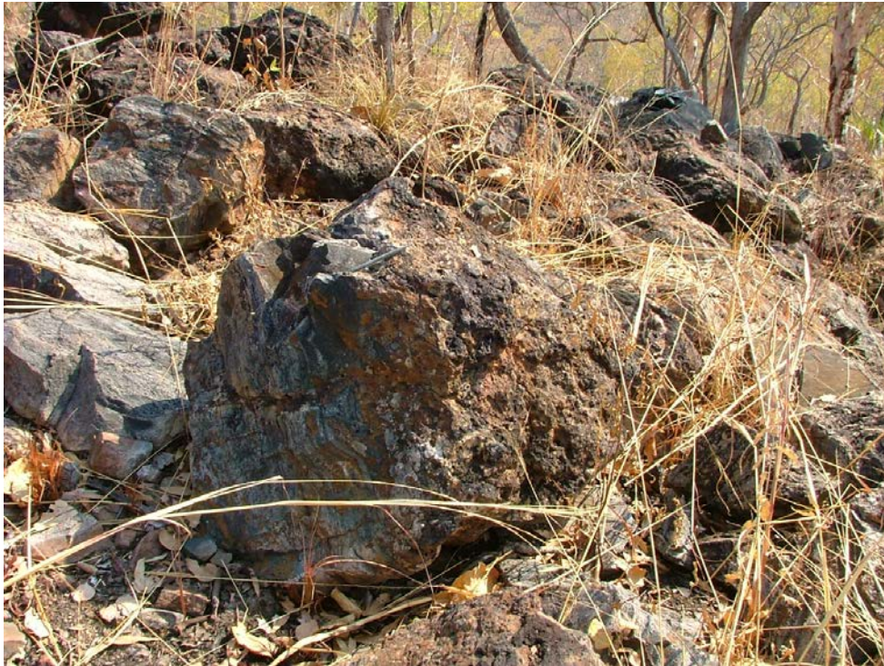
Figure 28: Breccia vein material (~0.5-1.0m wide) at Upper Mavis workings. Bedding plane vein striking NE and dipping 45^{\circ} to NW, near apex of NNE plunging anticline. A sample of this material (CC-002) returned assays of: 673 ppm Cu, 444 ppm As, 235 ppm Bi, 124 ppm Pb, 15 ppm Sb, & 0.07 ppm Au (with low values for Ag, Zn & Sn).
