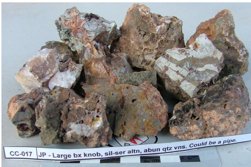
Figure 20: Example chips from sample CC-017 from the breccia pipe on SW side of Jason's Peak (see above). The sample returned: 0.47% As, 0.16% Pb, 370 ppm Sb, 72 ppm Bi, 95 ppm Sn, 1.2 ppm Ag & 0.19 ppm Au (with low Cu & Zn).
