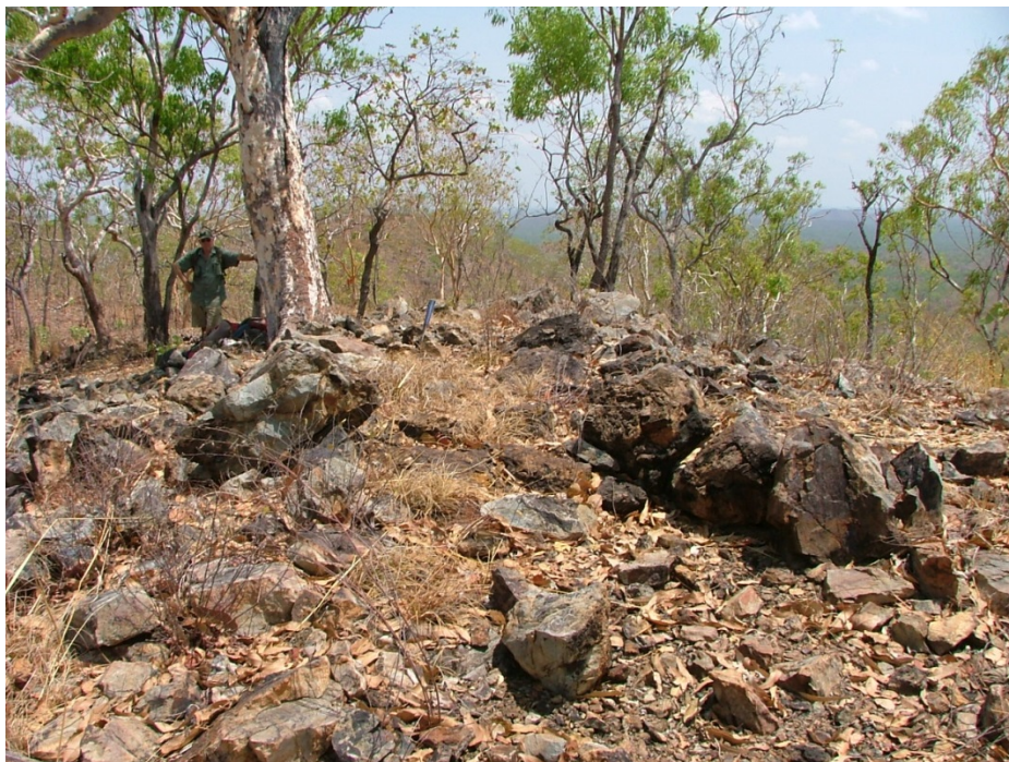
Figure 42: Narrow gossan-quartz veining in blocky altered metasediment (Sample 645925). The sample is anomalous in As, Pb, Sb & Cu, with 0.12% As, 658 ppm Pb, 83 ppm Sb, 237 ppm Cu, with weak results of 18 ppm Bi, 41 ppm Sn, 214 ppm Zn, 1.0 ppm Ag & 0.02 ppm Au.
