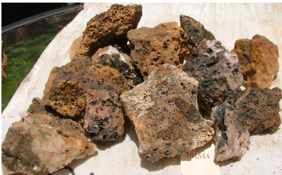
Figure 23: Example of sample 104544 from a ~0.5m brecciated and quartz veined fault in a small shaft on the north face of Jason's Peak. There are abundant disseminated boxworks (ex-pyrite?), massive gossan and irregular quartz veins. The assay results from this sample were: 0.57% Pb, 0.30% As, 782 ppm Sb, 167 ppm Bi, 394 ppm Sn, 2.2 ppm Ag, 0.04 ppm Au, 126 ppm Cu & 76 ppm Zn.
