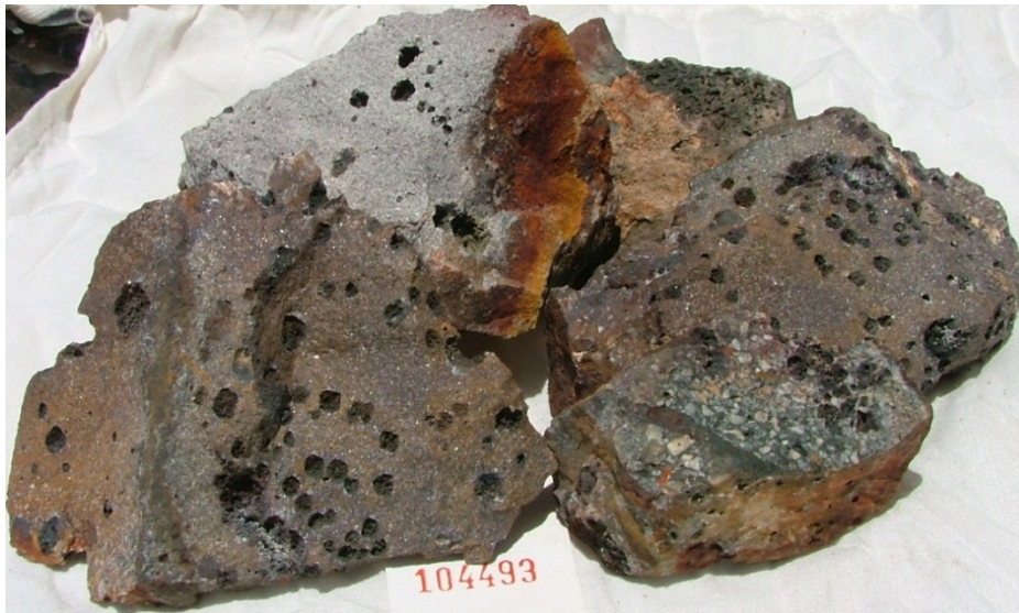
Figure 25: Example chips from sample 104493 of float pieces near the top of hill. The sample shows strong metasomatic (hornfels) alteration with abundant porphyryoblasts (ex-mafics?), along with siliceous breccia, quartz veining and possible sulphide boxworks. The assays show anomalous results of: 539 ppm Pb, 346 ppm As & 194 ppm Sn (other elements low).
