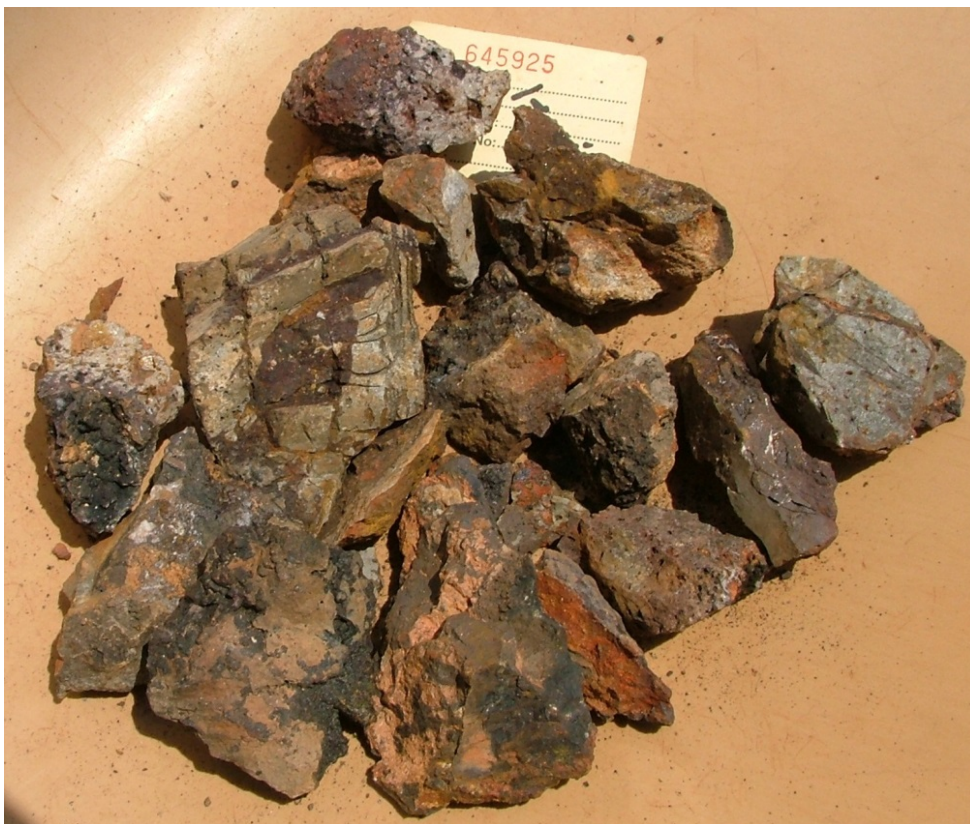
Figure 44: Sample 645925 (789822E / 8515454N – Figure above). Assayed 0.12% As, 658 ppm Pb, 237 ppm Cu, 83 ppm Sb, 18 ppm Bi & 1.0 ppm Ag (with weak Au, Sn & Zn).
