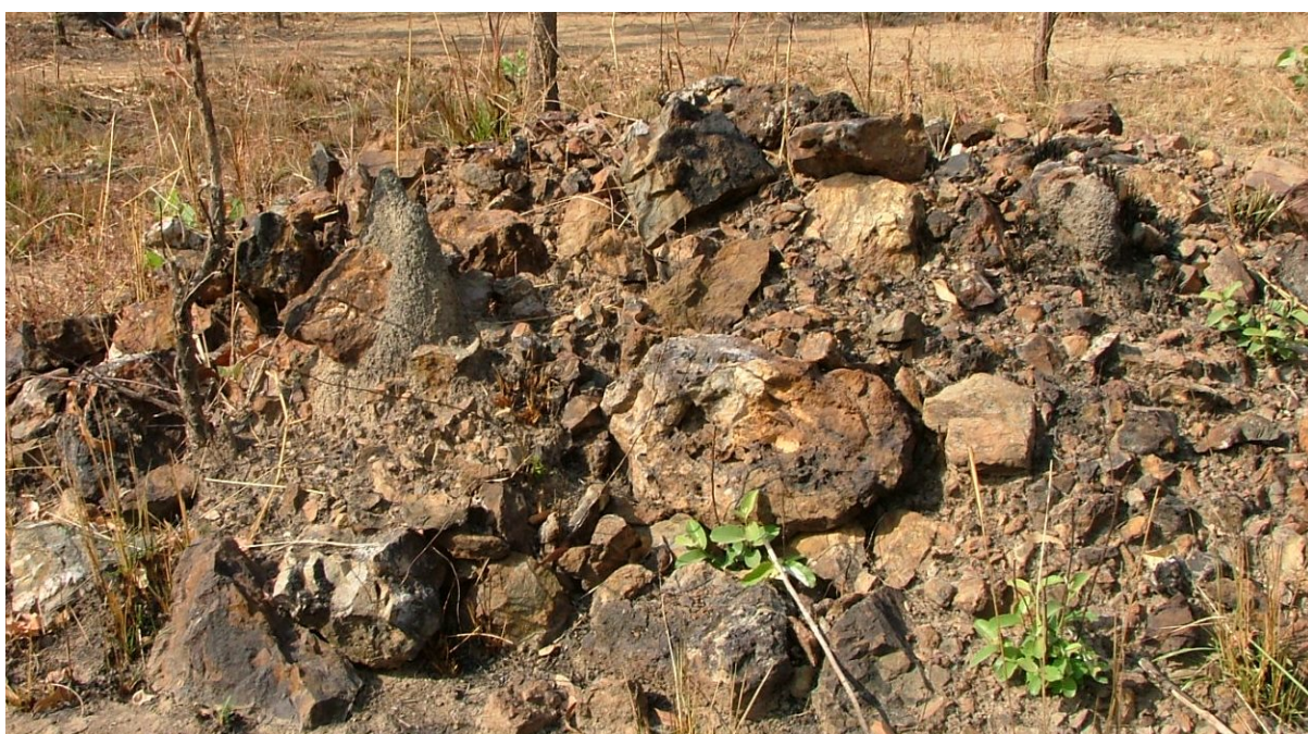
Figure 38: Hewson “stockpile” at base of hills, about 750m SW of the mine. The stockpile contains abundant large blocks of siliceous breccia with quartz and metasediment fragments, quartz veining and gossan infill with sulphide boxworks. Sample 645901 returned: 0.16% As, 706 ppm Pb, 225 ppm Sn, 103 ppm Sb, 24 ppm Bi, 2.1 ppm Ag, & 0.02 ppm Au (with relatively low Cu & Zn values).
