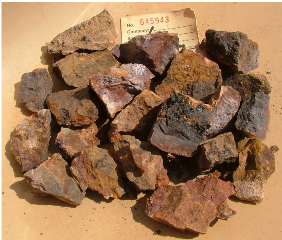
Figure 26: Example of chips from sample 645943 of a ~1m wide strongly altered vein zone on the lower north-east slope of the large altered hill north of Jason's Peak. This sample returned: 0.26% Sn, 477 ppm As, 309 ppm Cu, 207 ppm Pb, 43 ppm Bi, 16 ppm Sb, & 0.03 ppm Au (while Ag & Zn were relatively low). This anomalous geochemistry and strong alteration around this hill, extends the mineralised zone at least 700m north of Jason's Peak.
