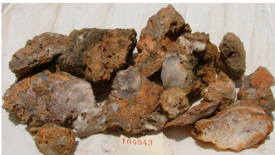
Figure 22: Example of sample 104543 from a ~1m wide brecciated quartz vein (fault) at Jason's Peak. The vein contains abundant FeOx boxworks & sponge filling voids in the brecciated quartz vein. The sample returned assays of: 1.12% Pb, 0.50% As, 661 ppm Sn, 275 ppm Sb, 261 ppm Bi, 336 ppm Zn, 100 ppm Cu, 11.5 ppm Ag & 0.06 ppm Au. This is a very high lead, arsenic, antimony, bismuth & tin system.
