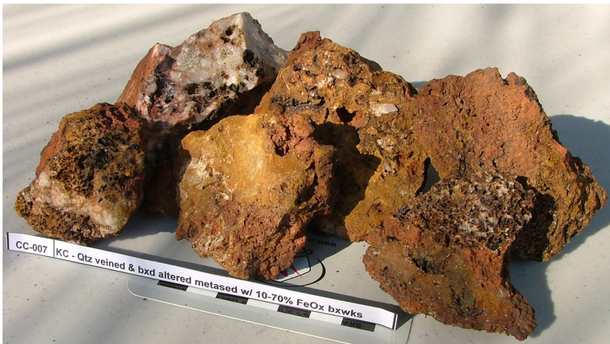
Figure 8: Kamas Cauldron breccia sample CC-007 with 0.73% As, 0.55% Sn, 103 ppm Pb, 35 ppm Bi, 68 ppm Sb & 1.1 g/t Ag (low Cu & Zn, and trace only gold).
