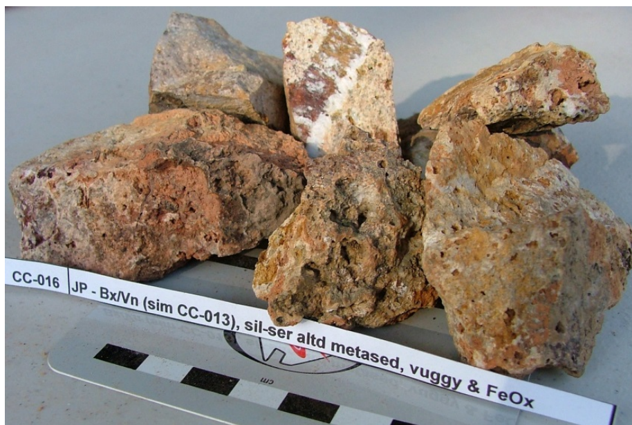
Figure 18: Example chips of the rock sample CC-016 (see above) which assayed: 1.64% Pb, 0.73% Sn, 0.14% As, 288 ppm Sb, 4.7 ppm Ag & 0.06 ppm Au (with weak Cu, Zn & Bi).
