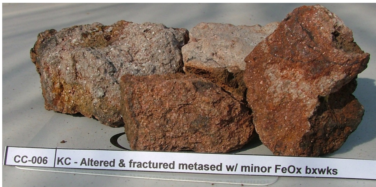
Figure 10: Sample CC-006 of altered metasediment breccia fragments in the centre of Kamas Cauldron. The altered metasediment (greywacke?) is now a medium-grained sericite-quartz rock with iron staining on fractures and occasional iron oxide boxworks along fractures.
