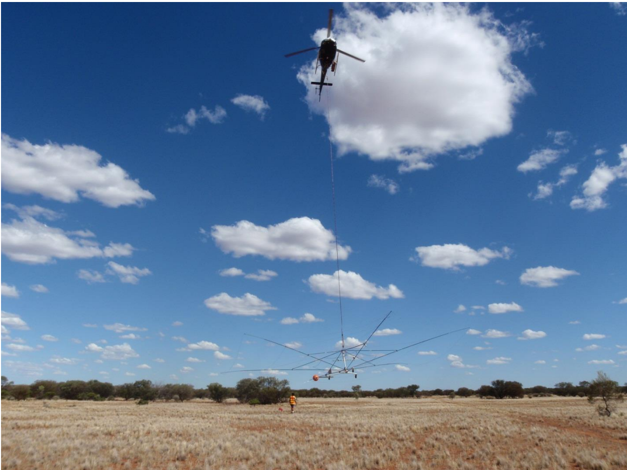
Figure 4: XTEM airborne geophysical system.
