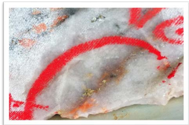
Figure 5. Drill core oriented to emulate drill angle. Flat-lying quartz veins with visible gold, from Buccaneer HGZ upper zone.
