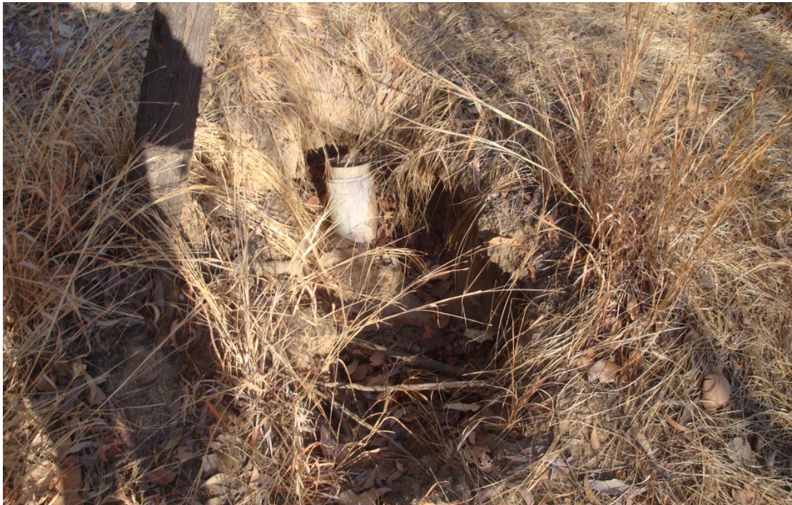
EXAMPLES OF DRILL COLLAR EROSION AT THE SANDY CREEK PROSPECT.
