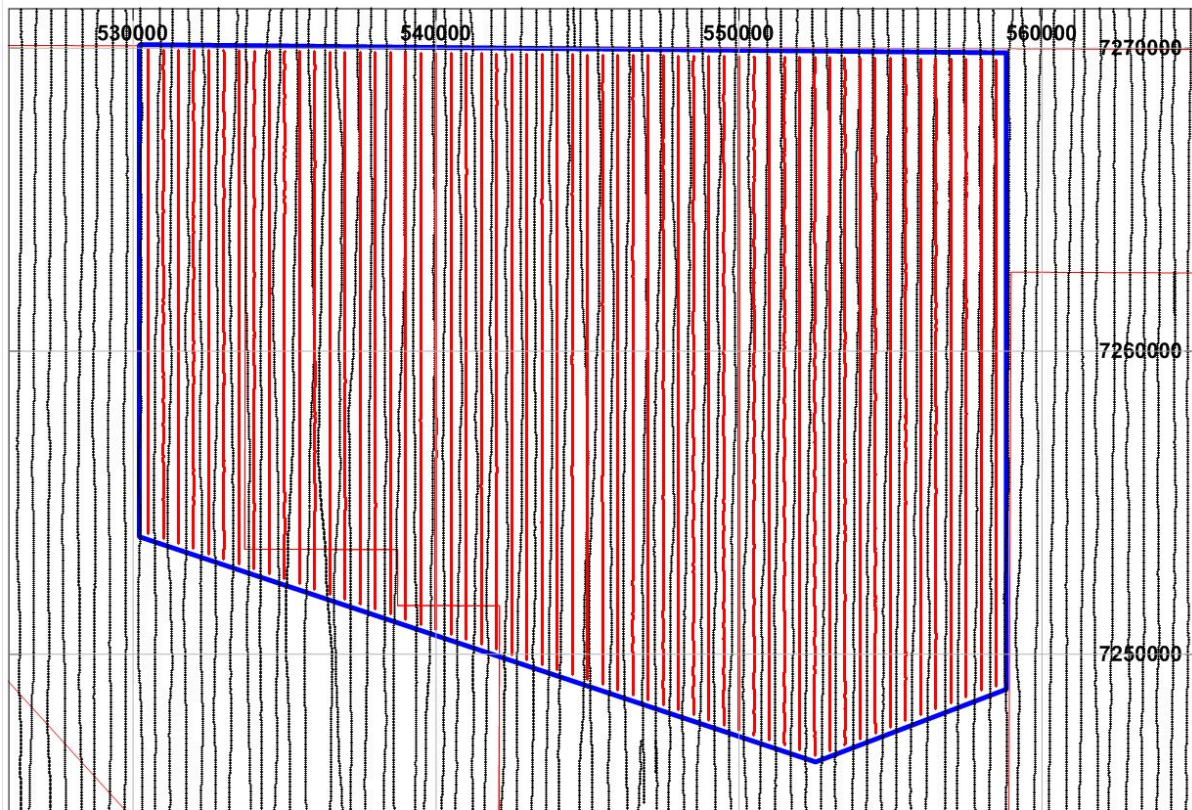
Figure 1. Flight path diagram for NTGS survey (black) and VTEM survey (red). The VTEM data were acquired using GPS navigation, and the flight lines are quite straight. The NTGS data were acquired using visual navigation from black and white photos. The flight path wanders; in places there are big gaps, and in other places lines cross.
