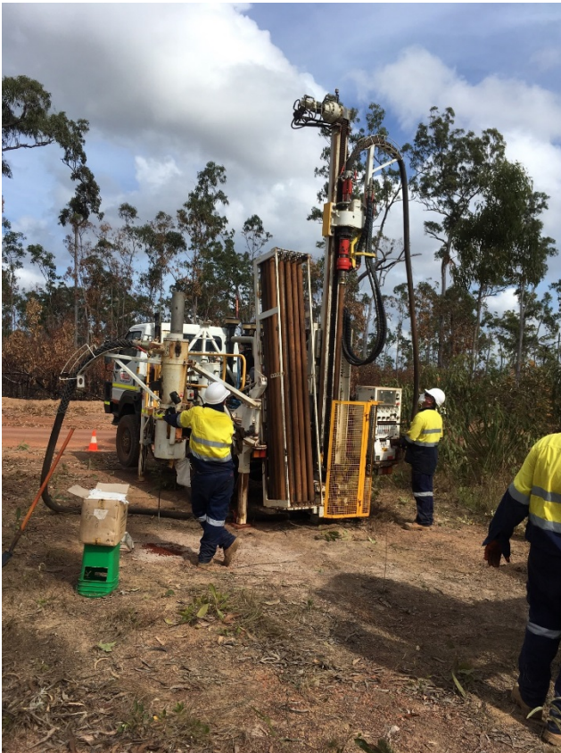
Figure 3 Wallis Mantis 100 drill rig working in Cato Plateau
