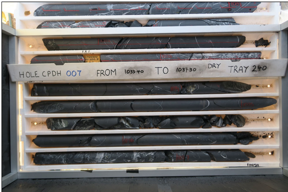
Figure 14 - Hole CPDH007, Barney Creek Formation, sulphidic carbonaceous siltstone
