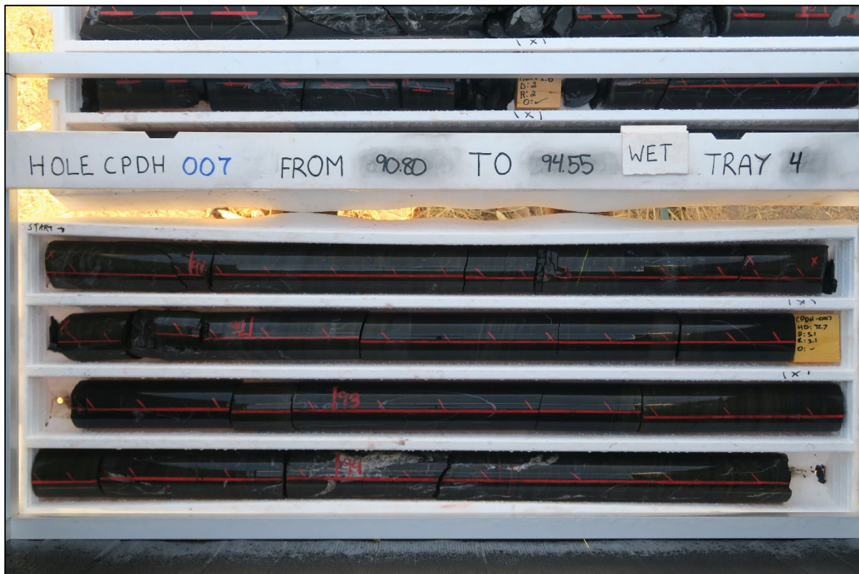
Figure 12 - Hole CPDH007, Lynott Formation, laminated pyrite in carbonaceous siltstone
