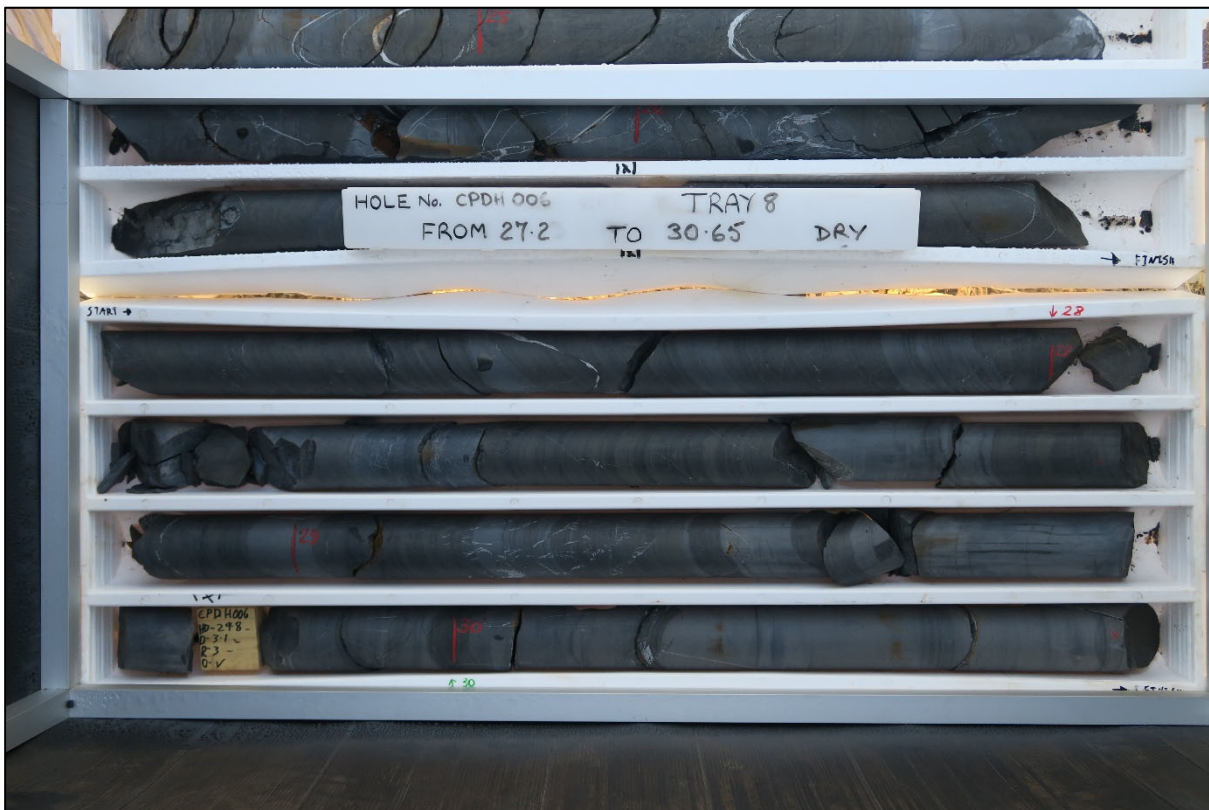
Figure 8 - Hole CPDH006, Lynott Formation, laminated pyrite in carbonaceous siltstone
