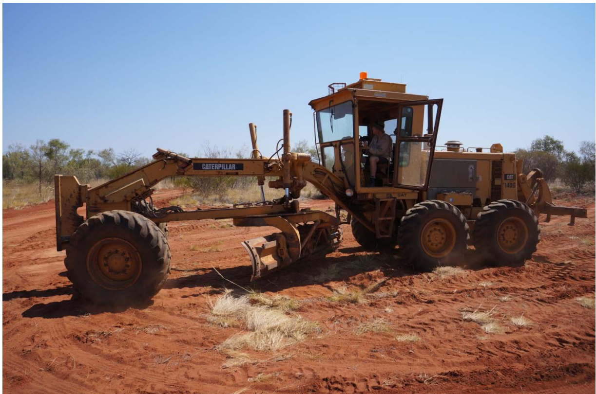
Figure 3. 140G Caterpillar Grader used to re-establish access tracks and clear new drill site.
