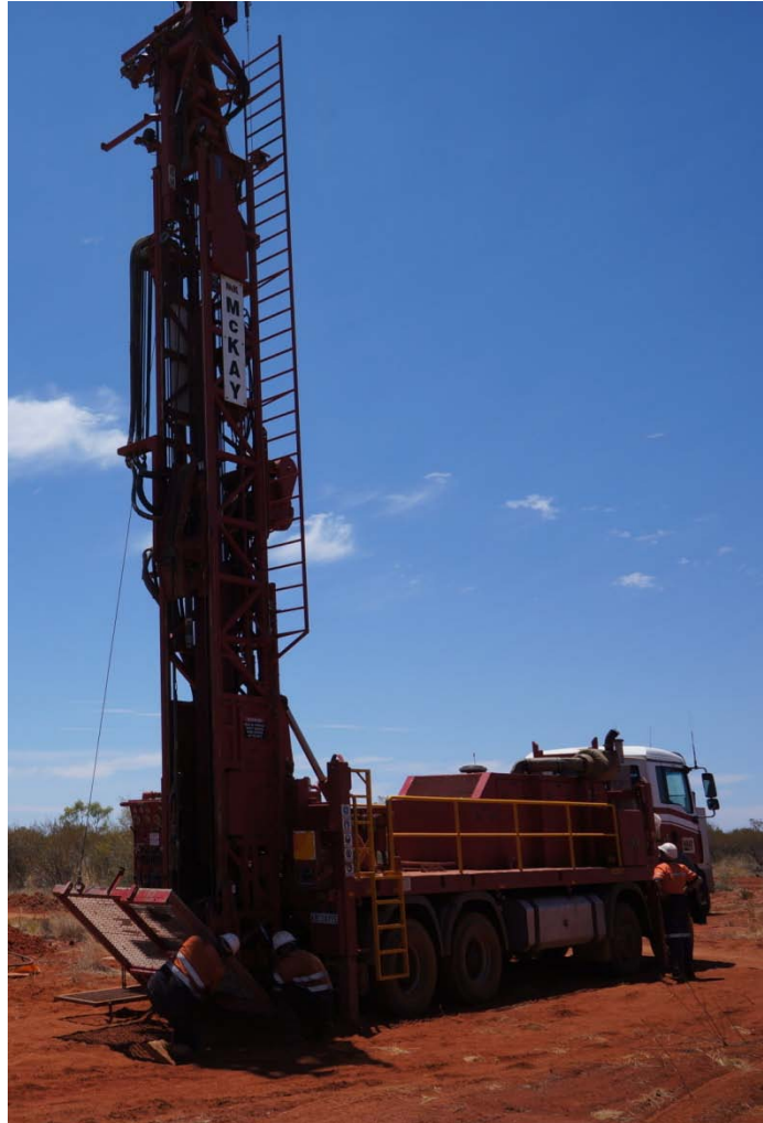
Figure 4. McKay Drilling Sandvik UDR 1200 diamond drill rig.
