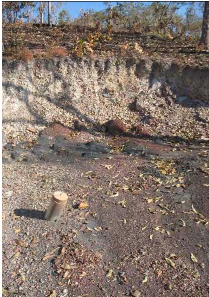
Figure 4 Plugged PVC Collar at MHRC 014
