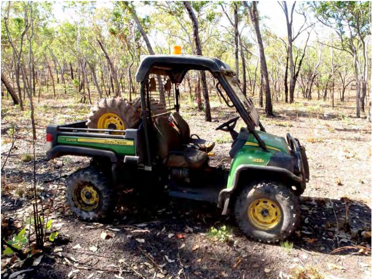
Photograph 5 The 'All Terrain Vehicle' used in the second half of the field programme. The vehicle is a John Deere 'Gator' 855D XUV 4x4.
