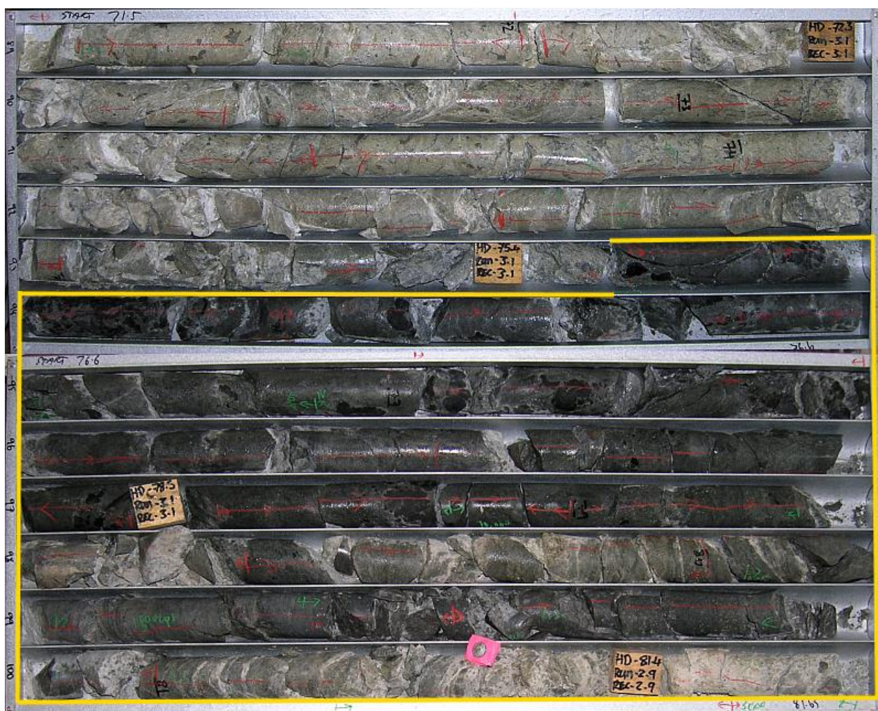
Figure 3: Core photographs showing the high grade mineralised zone in NAD4792 (6.3m at 7.23% U 3 O 8 , 1.9% Cu, and 0.66g/t Au from 75.5m – highlighted by the yellow outline) in contact with intensely sericite-pyrite altered schist (top). The chargeability anomaly.
