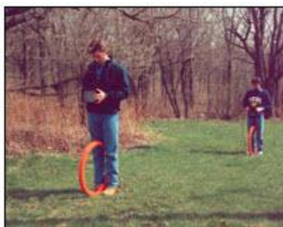
Figure24 – showing likely configuration of the EM34 coils for the Merlin surveys
