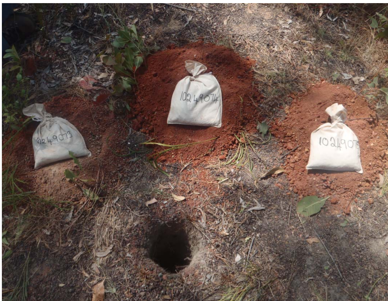
Figure 3 Photo of an auger site and the samples. Note the white material in sample 10249075 is saprolitic clay)
